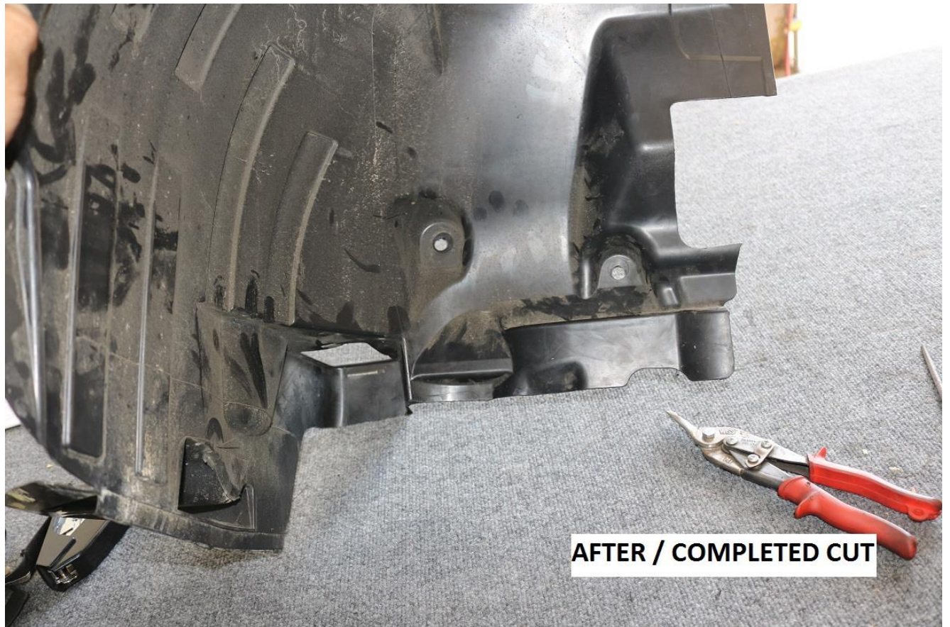
60) Trim the rear half of the fender liners as shown in the images above.
