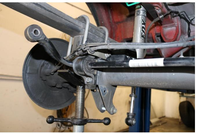
39) Install the 301501 rear sway bar links using the OEM sway bar link hardware removed in step 3. Torque the sway bar link bolts to 78 ft-lbs. (106 N.m).
