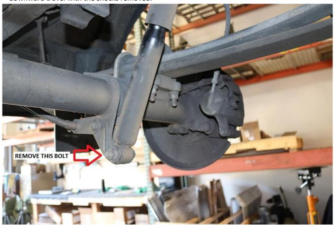
6) Remove the emergency brake cable brackets at the axle. Use a 13mm socket / wrench for removal. Retain this hardware as it will be reused. See image below
