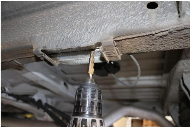
24) With both holes drilled, position the bump stop drop bracket in place and secure it to the chassis using the  $5/16-18 \times 1''$  long thread cutting screws included with the kit. Use a nut driver or drill with a  $\frac{1}{2}$ " bit adapter and a  $\frac{1}{2}$ " socket to install the screw. Try to keep the drill / driver as straight as possible when cutting the threads.
