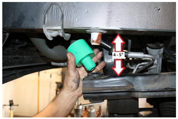
48) Install all 6 spacers in their corresponding locations and raise the sub frame into place.
