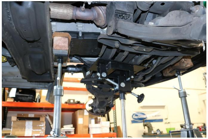
41) The wheel speed sensor wiring must be separated from the bottom clip on the chassis. See image below for reference.
