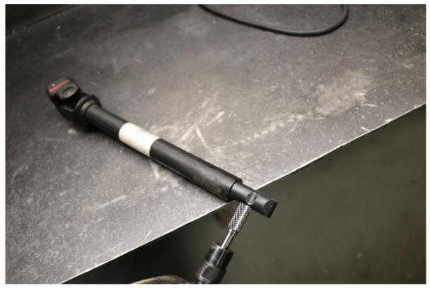
83) Once the pinch bolt can easily be installed, paint any newly exposed areas of metal to prevent corrosion. Assemble the steering shaft extension onto the steering shaft as shown below. Use a small dab of blue Loctite on the threads of the socket cap screw and torque to 18 ft-lbs (24N.m) using a 6mm Allen wrench.
