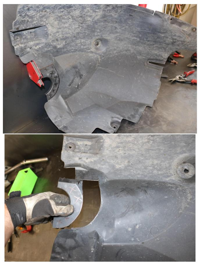
76) Again, if fitting 315/75/16 (35") tires, trim the rear half of the inner fender well liner as shown below. INSERT IMAGE OF TRIMMED REAR INNER FENDER LINER
