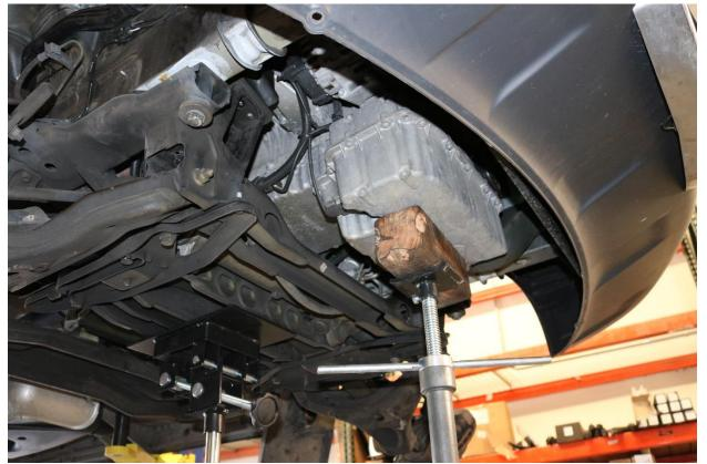
36) Remove the motor mount bolt on both the driver and passenger side with a 16mm socket / wrench.
