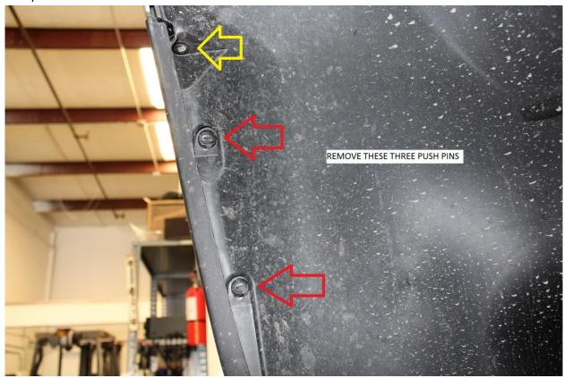
22) Note, the bottom two fasteners (denoted with the red arrows) are the same "cam style" fastener from step 5. The upper fastener (denoted with the yellow arrow) is a standard style push pin which can be
