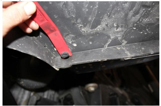
20) Using the same automotive trim removal tool, pry up under the head of the push pin body to fully removal the fastener.
