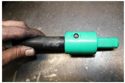
82) If the notch needs to be modified to allow for the bolt to be installed, use a small die grinder with burr bit or a 4-1/2" angle grinder with metal grinding wheel. Remove as little material as possible to allow fitment.
