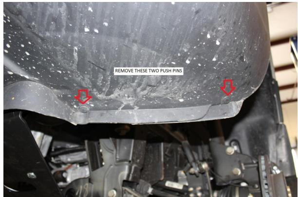
18) This style of push pin is a 3 step removal process. Begin by rotating the head of the push pin 90 deg so it cams out of the indent in the push pin body.
