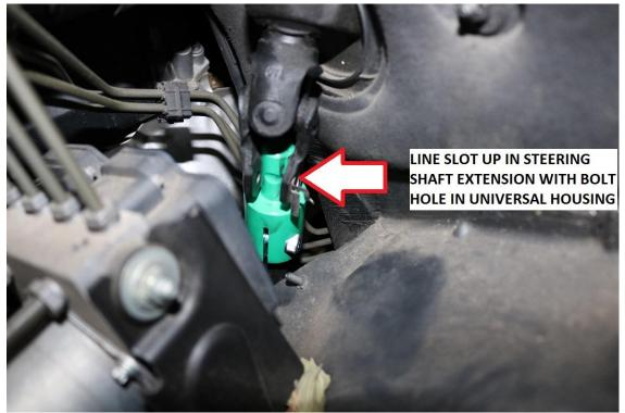
86) Install the bolt, retaining clip and nut removed in step 6 back onto the steering shaft. Use a 13mm socket / wrench and torque to 18 ft-lbs. (24 N.m)
