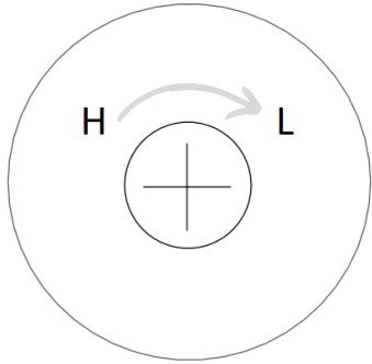
Turn the screw clockwise (**towards the L**) to increase the sensitivity of the pressure switch. Turn one half to one full turn. Continue turning until the correct calibration for dryer is achieved.
