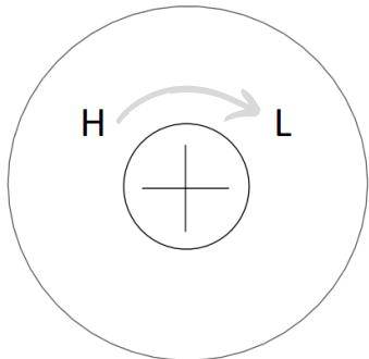
Turn the screw counter-clockwise (**towards the H**) to reduce the sensitivity of the pressure switch. Turn one half to one full turn. Continue turning until the correct calibration for dryer is achieved.
