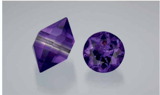
Figure 20. While synthetic amethyst, such as this 3.90 g crystal and 10.10 ct round brilliant, was not new in the last decade, advances were made in the use of FTIR spectroscopy to identify it. Photo by Robert Weldon.
