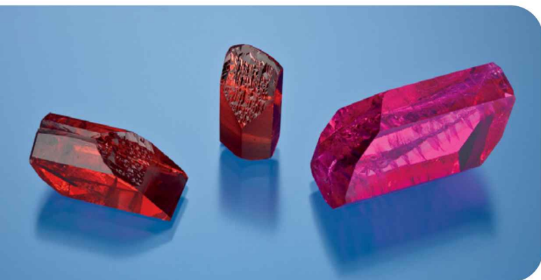
Figure 17. Manufactured in Moscow, these hydrothermally grown orange-red and pinkish red synthetic beryls derive their color from cobalt (left and center, 1.08 and 1.95 g) and manganese (right, 6.32 g) introduced into the nutrient solution. Photo by Robert Weldon.
