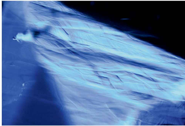
Figure 16. Like those previously produced in Russia, the Czech-Italian Malossi-manufactured blue beryls display characteristic roiled-to-angular structures or patterns of subgrain boundaries and intergrowths. Photomicrograph by Ilaria Adamo; magnified 25 \times .
