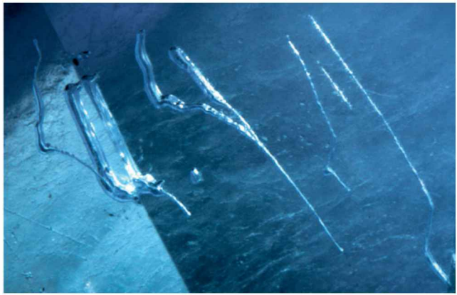
Figure 23. Significant amounts of neodymium and strontium were detected in this unusual 3.03 ct color-change synthetic apatite. Magnification (right) revealed features that indicated synthetic origin, such as these elongated gas bubbles. Left photo by Robert Weldon; right photomicrograph by J. I. Koivula, magnified 30x.
