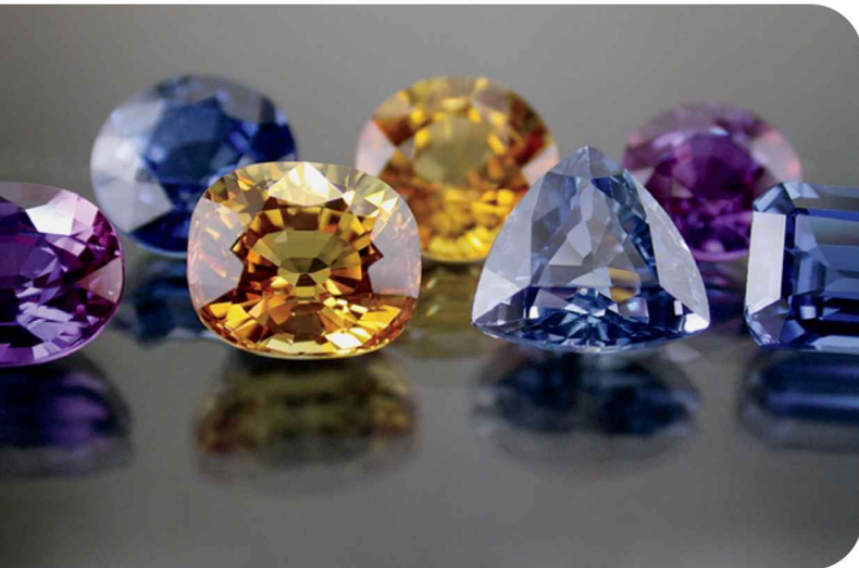
Figure 24. Purchased over the internet, these were advertised as heat-treated natural sapphires, but all turned out to be flame-fusion synthetics (4.5–7.0 ct).
