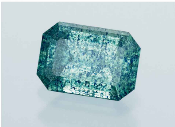
Figure 11. This 0.91 ct bluish green flame-fusion synthetic sapphire displayed a bodycolor and inclusions the GIA Laboratory had never encountered before. Photo by Robert Weldon.
