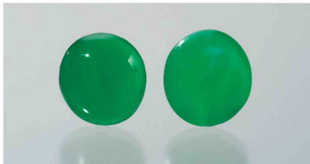
Figure 18. During the past decade, General Electric grew extremely high-quality synthetic jadeite, as illustrated by these two cabochons (5.20 and 6.73 ct). Photo by Robert Weldon.
