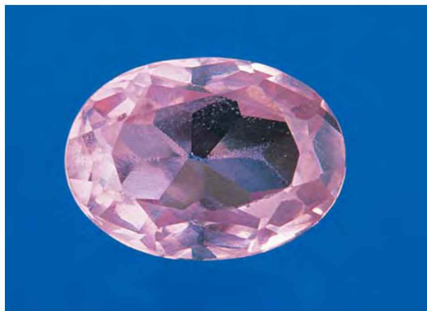
Figure 13. This attractive titanium-doped Czochralski-pulled synthetic pink sapphire, here 1.20 ct, has been referred to as “Ti-sapphire.” Photo by Maha Tannous.
