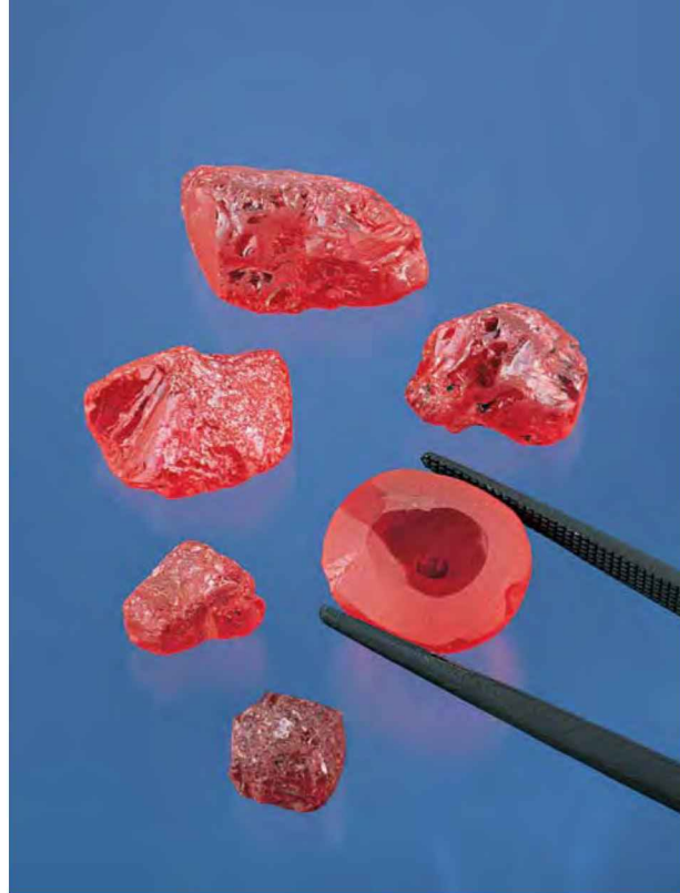
Figure 33. All of these pieces of tumbled rough and cobbled material (3.79–15.17 ct) were purchased in Vietnam as ruby, but only the smallest and darkest piece of rough (pictured at the bottom) proved to be natural. All of the others were flame-fusion synthetics that had been fashioned to mimic their natural counterpart. Photo by Shane F. McClure.
