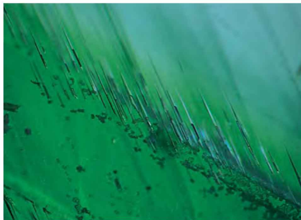
Figure 16. This dense pattern of nailhead spicules and chrysoberyl crystals, usually located near the seed plate, is typical of that seen in the hydrothermal synthetic emeralds produced in Guilin, China. Photomicrograph by John I. Koivula; magnified 30×.
