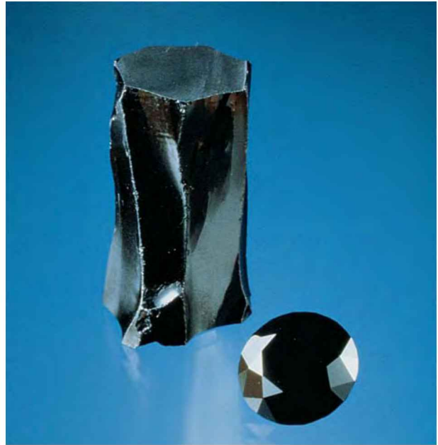
Figure 30. Black, nontransparent cubic zirconia from Russia was used as a black diamond simulant. The faceted sample weighs 6.60 ct. Photo by Shane F. McClure.
