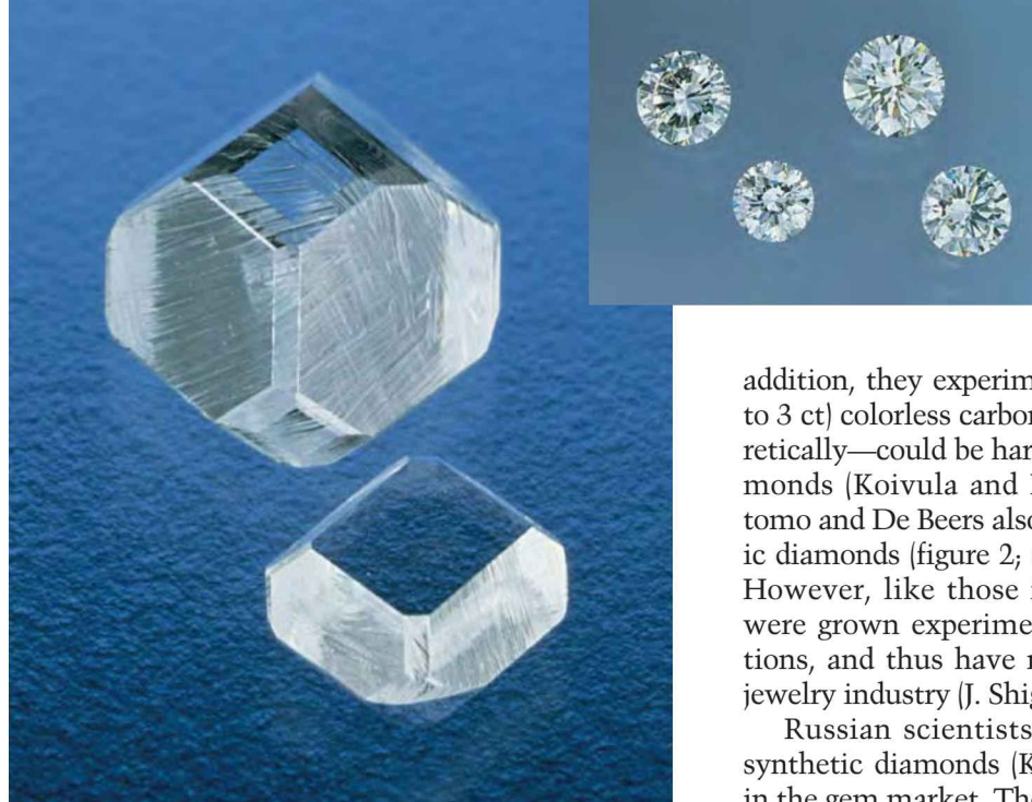
Figure 2. Both Sumitomo and De Beers grew near-colorless synthetic diamonds for experimental purposes. The faceted De Beers near-colorless synthetic diamonds shown here (inset) weigh 0.41 to 0.91 ct. The two Sumitomo synthetic diamond crystals (0.23 and 1.25 ct) exhibit a cuboctahedral form, which is typical of synthetic diamonds from all known manufacturers. Left, photo © GIA and Tino Hammid; inset photo © GIA.
