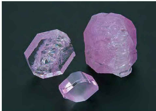
Figure 20. Large amounts of transparent synthetic pink quartz (here, 1.95–16.06 ct) also entered the gem market during the past decade. Manufactured in Russia, this hydrothermal synthetic was sold as Flamingo Quartz. Photo by Maha Tannous.
