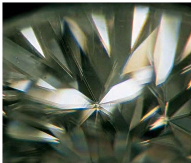
Figure 5. Synthetic moissanite is fairly easy to identify with a microscope or a loupe. When you look through the crown, doubling of the back facets readily reveals the doubly refractive nature of this diamond simulant. Photomicrograph by John I. Koivula; magnified 20×.
