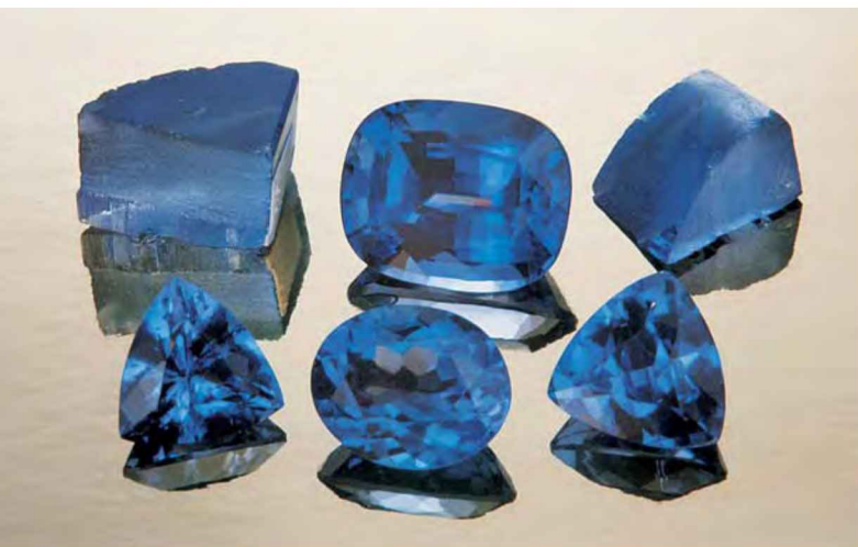
Figure 24. With their color and strong pleochroism, these cobalt-doped synthetic forsterite samples closely resemble tanzanite. The largest cushion mixed cut weighs 6.15 ct. Courtesy of Tom Chatham; photo by Maha Tannous.
