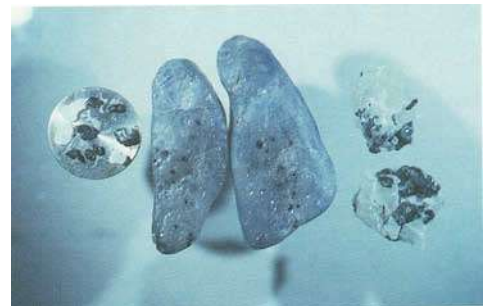
Figure 4: Sapphire samples obtained from a source in Switzerland (Source C, see text) with eye visible inclusions. On the right, a rock fragment collected at the mines is shown. The section on the left demonstrates how the minerals were prepared for SEM-work.
