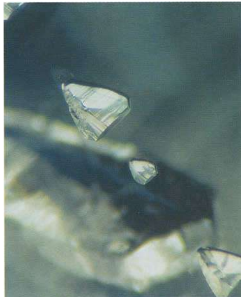
Figure 13b: Sapphire from Source A: negative dipyrramids n(22\bar{4}3) aligned along the c -axis, and blue colour phantom. 40x.
