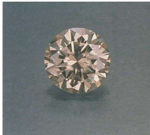
Figure 6: A synthetic moissanite, the most recent diamond substitute (1.68 ct, colour about G on the GIA diamond scale). Photo courtesy of C3 Inc. of Raleigh, NC, USA, which is introducing this material in 1997.
