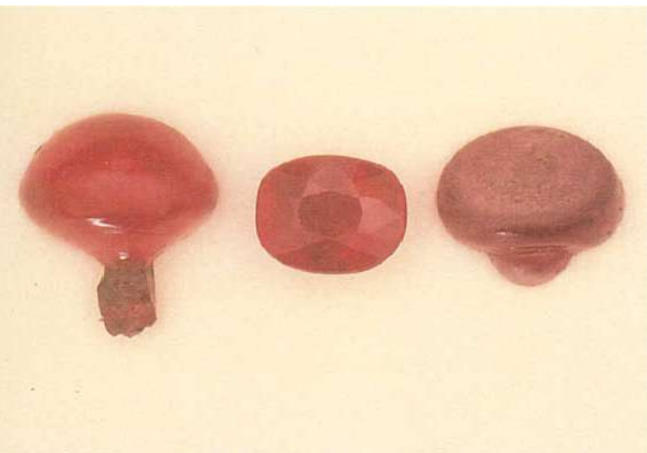
Figure 3: 'Geneva' synthetic ruby produced about 1885 and sold as natural at that time. Photo copyright Kurt Nassau.
