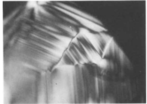
Fig. 31. Growth structures in Russian flux-grown synthetic emerald; planes parallel to the hexagonal prism m and m' \{10\bar{1}0\} form an angle of 120^\circ , smaller planes parallel to the prism a (11 \bar{2} 0) are also present. View parallel to the c -axis. Crossed polarizers. 20x.
