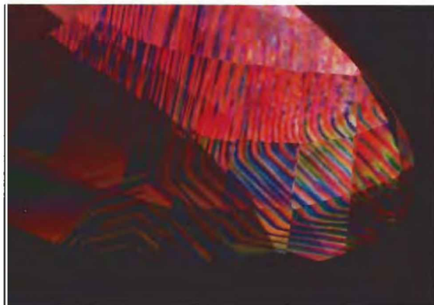
Figure 8. The difference between the twinned natural (left) and the untwinned synthetic (right) amethyst is clearly seen looking in the optic axis direction of each under crossed polarizers. Photos by Shane F. McClure.
