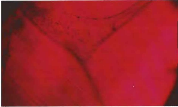
Figure 5. A flux healing process was used to induce this "fingerprint" in a Verneuil synthetic ruby. Also note the curved striae characteristic of the Verneuil flame-fusion process. Photomicrograph by John I. Koivula; magnified 45 \times .
