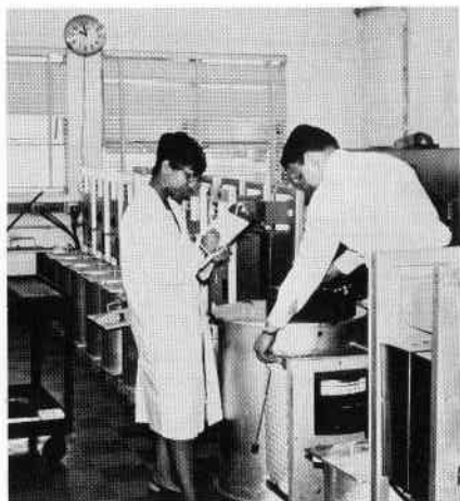
Figure 8. Hydrothermal synthetic emerald growth at Linde, about 1965. Courtesy of Union Carbide Corp.
