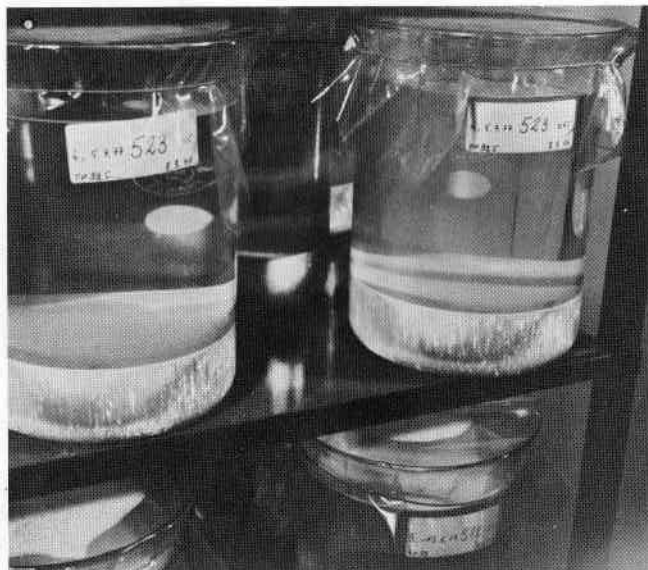
Figure 9. Gilson Opal during its one-year settling period. Courtesy of Ets. Ceramique Pierre Gilson.
