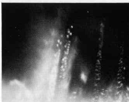
Figure 5. Reflections from plate-like inclusions (x100).
