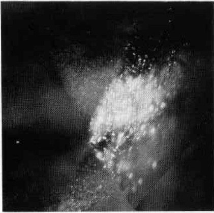
Figure 6. Reflections from plate-like inclusions (x25).
