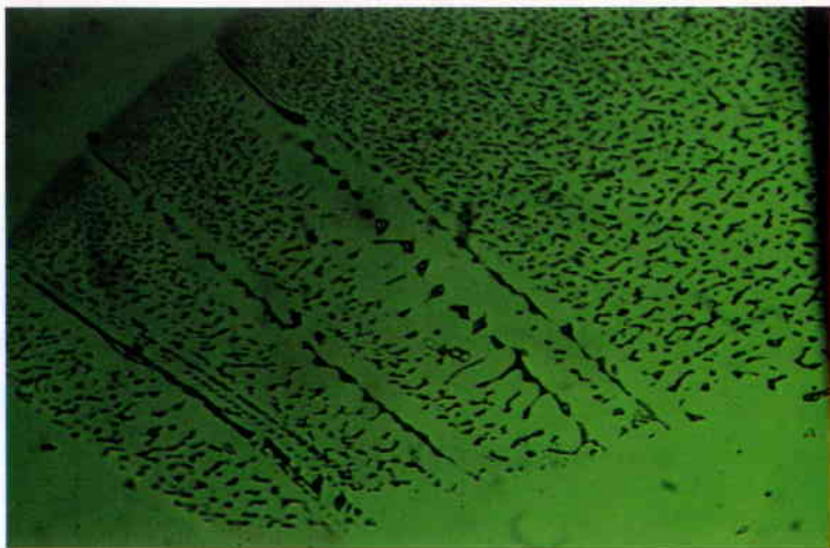
Figure 6. A section of a "fingerprint" inclusion, i.e. a partially healed fracture marked by a system of intercommunicating channels of residual liquid (40x).
