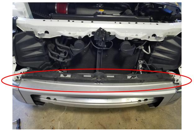
Next, we'll remove the entire front bumper assembly by removing these 6 14mm nuts.
