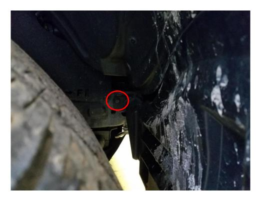
Remove your upper grille. There are 4 10mm screws and two push pins holding the top on. The bottom is a plastic push clip built into the grill. It attaches to the body pieces beneath the headlights near the bottom left and right edges on the grille.
