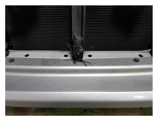
Using that clip I mentioned for you to hang on to, reattach the sides by the fender liners. Your bumper will gently hang in this position while you install the bumper.
