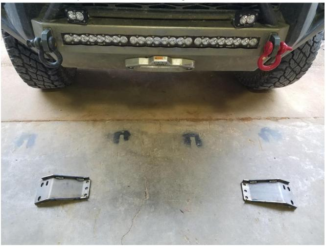
Slide these into place from up and under and tighten the 3 vertical bolts first, generally square to the bumper. The adjustability in the slots should allow for plenty of movement for the perfect alignment, however you can loosen the 3 vertical bolts for even more adjustability up or down on each side.
