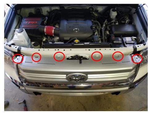
Remove this center bracket with a 10mm socket.
