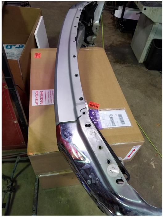
Next, we need to remove the aluminum crash bar from the bumper assembly. To do that, begin by unbolting the side brackets from the bumper until all you're left with is the aluminum crash bar and side brackets.
