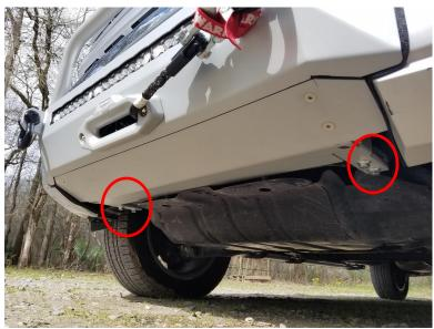
Slide the bumper onto the truck and ONLY secure it using the (4) m12 bolts from below and (1) m10 nut on each inner side of the mounting pad. Leave the 3 bolts in a vertical line on each side unbolted for now.
