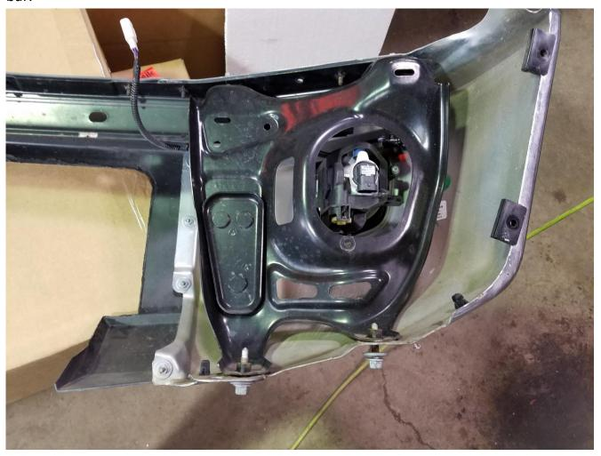
Also, reattach the fender liners back to the oem assembly. We'll be using that clip location to help us secure the bumper for a few minutes while installing the Slimline hybrid.
