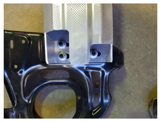
Reattach the side brackets back to the bumper assembly. Discard the aluminum crash bar.
