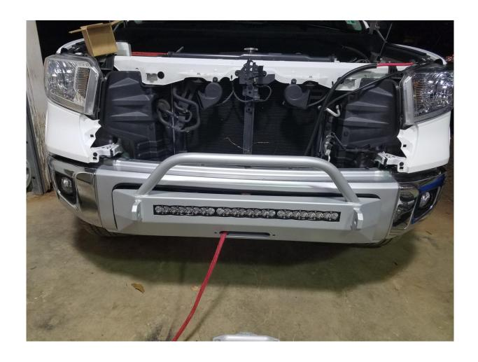
Now, you'll need to install the supporting side brackets that hold the oem bumper into place. The side brackets supplied utilize the same 3 holes that we left unbolted on the bumper itself. The other 3 holes in a triangle attach to the brackets that are already bolted to the oem bumper. They are slotted to allow for maximum adjustability.
