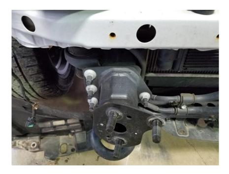
Carefully place the modified bumper assembly back into position on your Tundra. To hold it in its general location, use the provided zipties to secure it at the middle like this.
