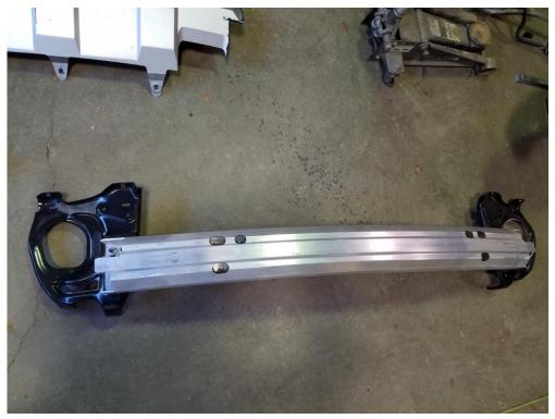
Remove the side brackets using a 14 mm socket.
