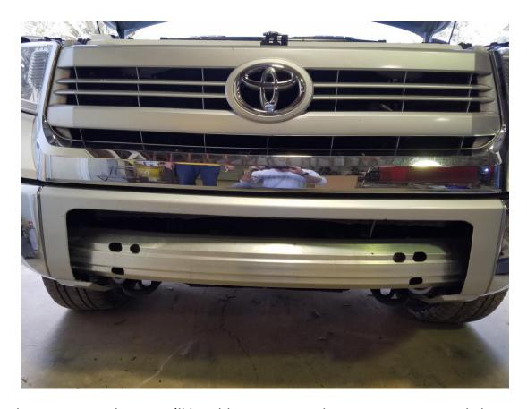
Once the cut is complete, you'll be able to remove the center section and clean up any ragged edges left with a razor knife.
