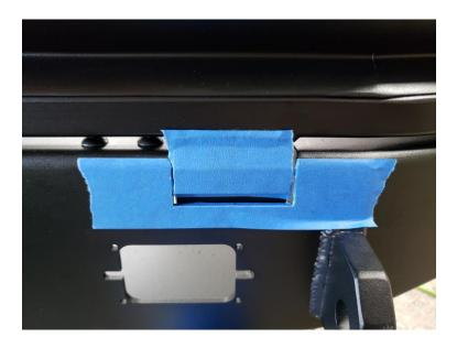
Gently insert the TrailGator into the hinge holes. It will rest in the fully open position with no assistance.
