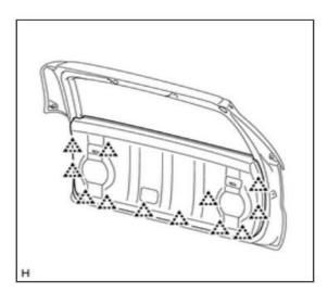
Remove the strap cover and also the 10mm bolt that secures the strap to the door. Gently pop the panel off the door at the indicated locations. Lift the panel off the rear door by detaching the (9) claws around the glass weather-stripping as shown below.
