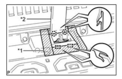
Remove the driver and passenger side mud flap.
