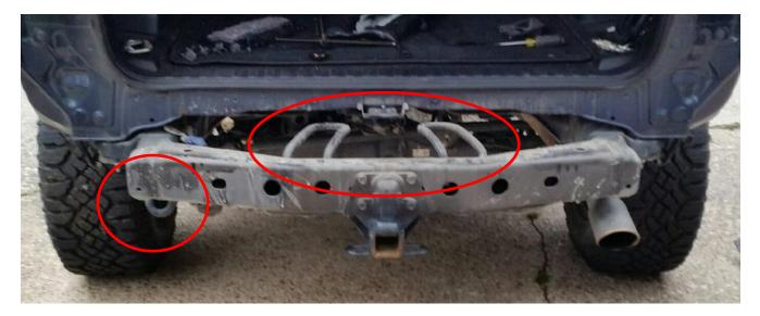
Remove the towing wire harness from its oem location and relocate using the supplied spacer to the rear of the frame as shown with supplied m8 bolt. There will be a captured nut in the frame that can be used for this purpose.
