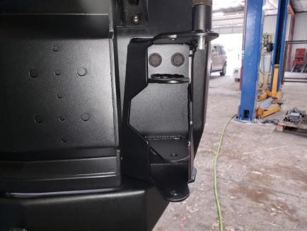
Install the 4 oil-impregnated bronze bushings, top and bottom of each bolt location. Install the locking pin ramp. Torque to 8ft/lbs.
