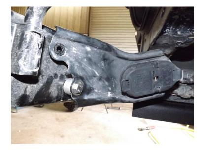
Ensure that the factory welds are smooth across the frame rails. Grind down any welds that prevent the 3/8" brackets from seating flat against the frame.
