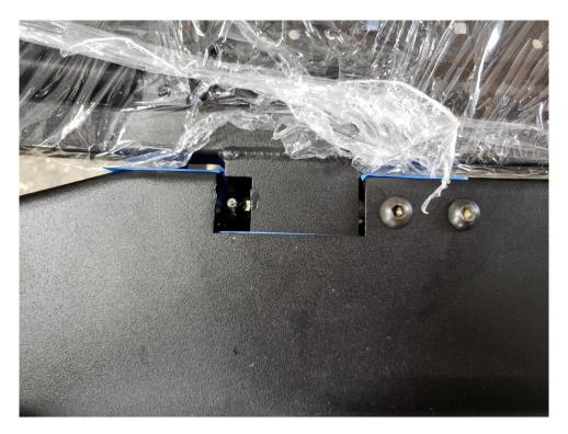
Loosely install the TrailGate latch stops and rubber bumpers on both sides of the bumper using the provide 3/8" black button head screws.
