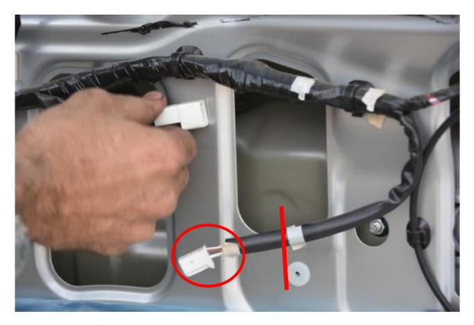
You will basically be extending these (4) wires so that they reach the new camera location in the swing arm. The plug that is cut from the OEM harness (circled in red) will be used again at the new camera location. This allows for replacement of the camera itself by just unplugging the connector.
