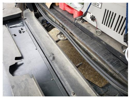
Gently pull back the rubber molding around the rear door.
