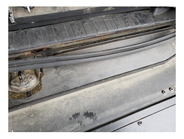
Lay the bumper to truck cover plate into place.
