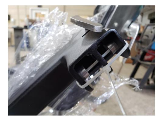
Carefully slide the swing arm into position and use the provided 3" long 7/16" bolts and locking nuts. Don't apply too much torque, as the swing arm will be more difficult to open and close than it needs to be.
