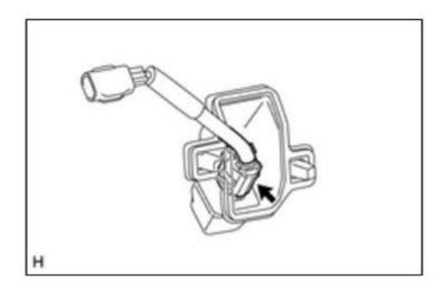
Remove the oem camera from the plastic housing. Using the small oem screws that are found in the back of the camera, mount the camera to the relocation kit bracket .
