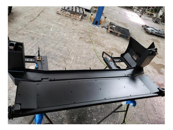
Install The Zirk fitting pointed up and slide the ball bearings into the tailgate side of the hinge. Insert the hinges from inside the bumper with the installation handle at the top.
