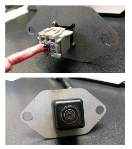
Mount the camera bracket to the license plate bracket provided in the relocation kit.
