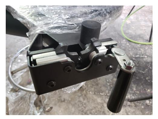
Close the swing arm and align the slam latch pin to be directly in the center of the slam latch. Adjust the rubber bumper to provide cushion while not inhibiting the catch mechanism. **The weight of a spare tire may necessitate** slam latch pin adjustment.
