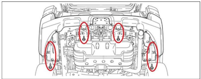
Remove the remaining (8) 10mm bolts and apply protective tape to the paint on the body along the seam line. Gently begin unlatching the plastic clips along the body of the truck to completely remove the bumper cover. Pull the panel at the rear of the wheels down and outward. The panel will pop right out. Do the same on opposite side of the vehicle, then work loose and pull panel outward from the tailgate area. Look to the image below for clarification on latching system.
