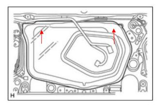
(NON PREMIUM VEHICLES) Remove the back door lock cylinder using a 10mm socket to remove the 2 nuts.
