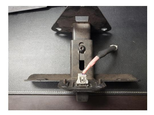
Cut the OEM wiring harness nearest the plug still attached to the rear door to splice in the lengthened SSO harness. It is important that you make this cut so that there are (4) wires and not (3). One of those wires is a shielded cable that splits off into (2) near the electrical connector. Once again, make sure you make the cut where there will be (4) wires on both sides of this cut. You may need to trim away some of the black protective loom.
