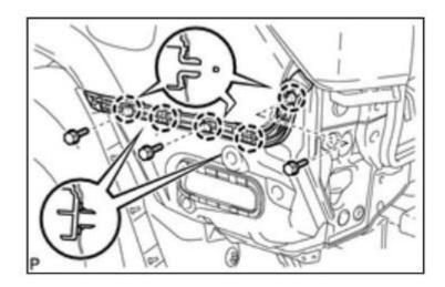
Remove the tail lights and the plastic bumper retainer under the tail lights. Access the tail light bolts from inside the truck behind the tail light access panel. Remove the 10mm nuts with an extended socket.
