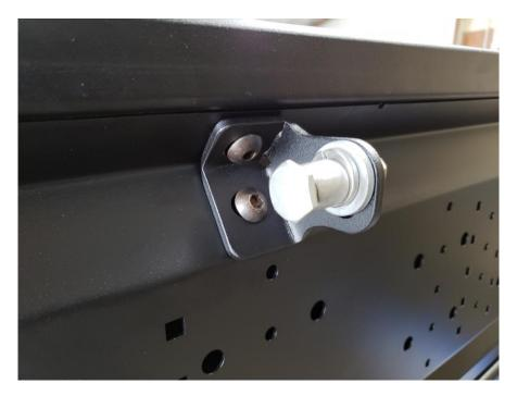
Install the slam latch, cover, handle, and rubber stop as shown. Use the black 1/4"-20 x 1.25" long bolts. Torque to 12-15 ft/lbs.
