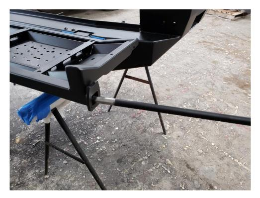
Slide the delryn bushings over each end and into the Trailgator. You'll want approximately 1" protruding from both ends.
