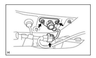
Remove the outside trim piece to finally access the rear view camera.
