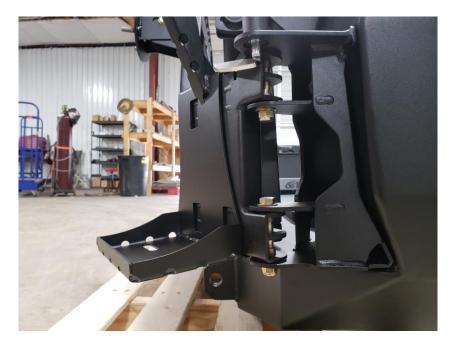
Loosely install the slam latch locking pin as shown.
