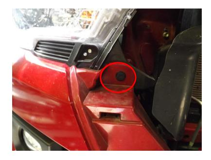
Remove every 10mm bolt on the underside of the OEM bumper cover.
