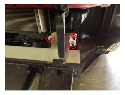
Remove this center frame rail from the truck.
