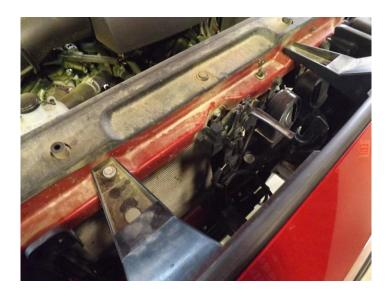
First, remove two the 10mm bolt heads holding the upper portion of the grille to the body of the truck. Also, remove the push pins near each headlight with a flat head screw driver by pulling up on the center section first, then pulling the clip out completely
