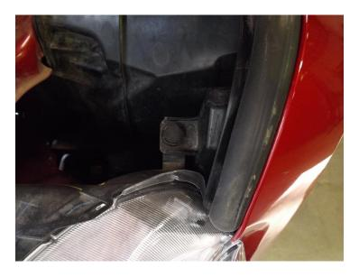
After removing the upper fasteners, you will also need to remove the remaining lower push in clips holding the grille cover onto the truck. You will find these clips all along the bottom of the grille. With a little finess and steady but gentle pulling and maneuvering you should be able to work the grille free. Pull and wiggle from the bottom to unseat these clips. You could also reach from behind the grille to unseat each of them individually.
