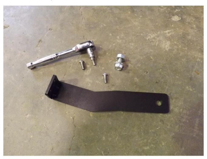
With all bolts still relatively loose, align the Slimline Hybrid as well as oem plastic bumper cover for best fitment. Once fitment has been found, slowly tighten all m10,m12 and also the wing bracket bolts. Tighten m10 nuts to 75 ft/lbs and m12 bolt to 110 ft/lbs.
