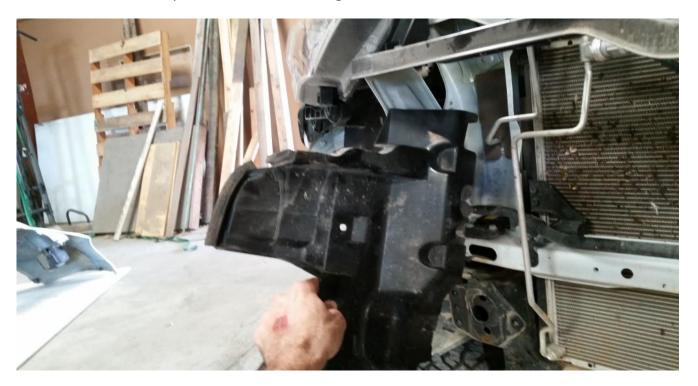
Using 10mm/Phillips screws and pushpins, reinstall the OEM bumper back on to the truck. Some original mounting points will be unavailable, but use as many as possible. Install the grill and all of the pushpins from the top as well as the Phillips head screws into the fender wells and top of grille. **Go in reverse from instructions on pages 3-8.**
