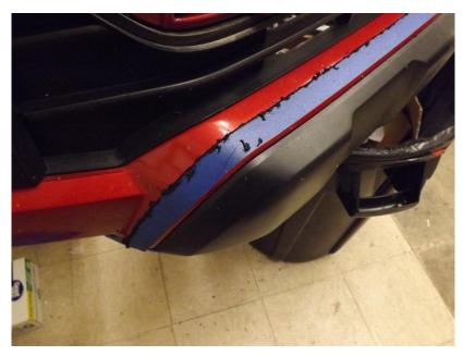
After making the initial long cut, cut down each side following the outside edge of the painters tape, but leaving enough oem bumper to install the supplied edge trim. You should now be left with a piece like this:
