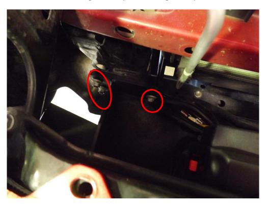
Also install the supplied m12 bolts into the radiator support through the leg on each side of the Slimline bumper. The crash bar houses the captive nut for this bolt. Be certain it is in place.
