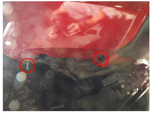
Remove the remaining clips and fasteners connecting the fender liner to the front bumper cover, using a 10mm ratchet for the top screw and a flat head screwdriver to turn and pull out bottom plastic clip
