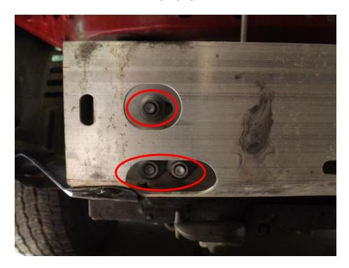
Remove the 8 - 14mm flange head nuts holding this section to the frame rails.
