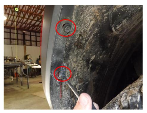
You also need to gently detach the fender trim from the front bumper. Don't pull to hard to far back, it is 3M taped further back and will NOT re stick.
