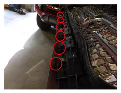
After removing the grille, remove the remaining push pin clips holding the bumper onto the truck from the front.
