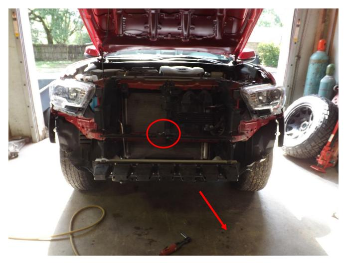
When the OEM bumper has been removed, you'll expose the cross beam that joins the frame rails together. Loosen one leg of the aluminum cross section (14mm), but do not remove.
