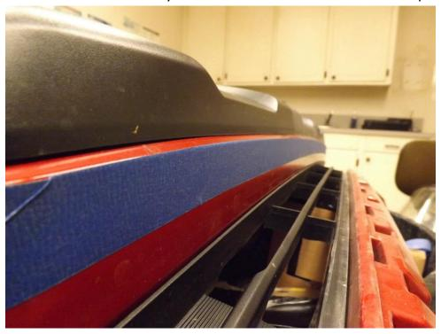
After rounding each corner downwards, trail it straight down onto the black plastic lip. Use a new piece of tape to now connect the previous piece of tape laid to a bend line indicated below. It will taper to less than an inch at this point from the original edge.
