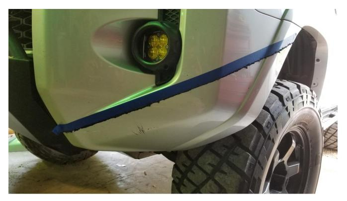
Once the cut is complete, remove the two 10mm screws from the fender liners to release the cut plastic. Leave the top 10mm screw in place.
