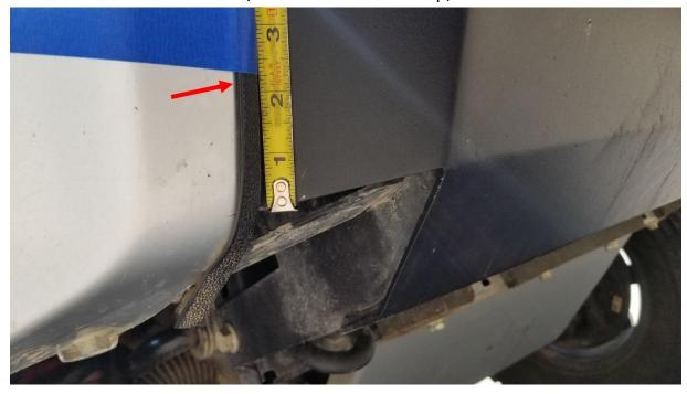
Using this newly created line, carefully place your 1" wide painters tape as straight as possible. **The bottom edge of the tape should be used to line up the marked points.** It is helpful to utilize the straight edge under the fog light as a guide when connecting each newly created point.
