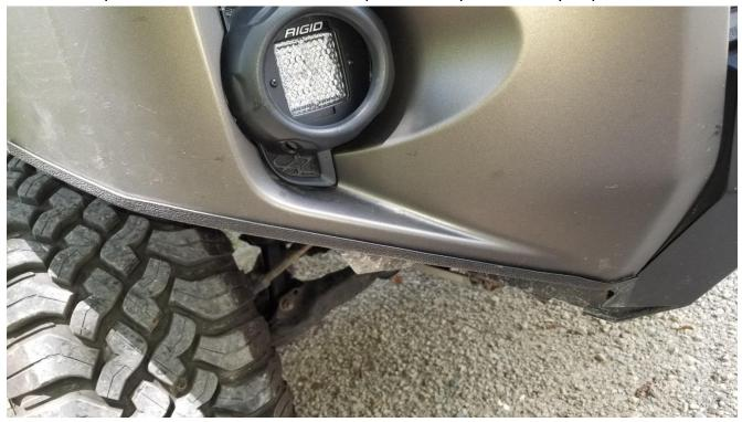
Reinstall the Stage 2 High Clearance on both sides for the final fitment. Use the provided 3/8"-16 flange nuts and the 3/8" bolts you removed from the side brackets earlier.
