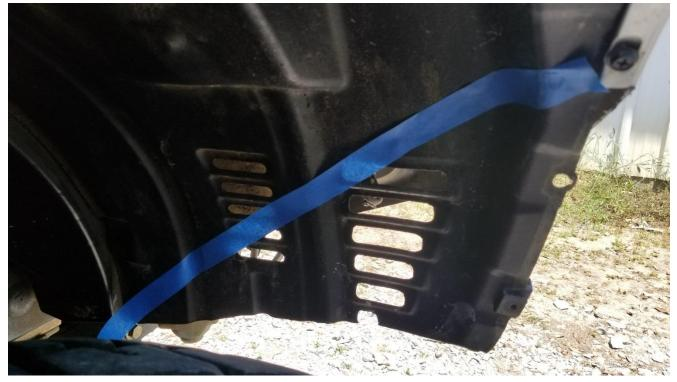
Remove the m12 (17mm head) from the lower radiator support. Lift the High Clearance side protection into place to mark and drill for new holes. (New Slimline Hybrids already have these holes in place, no drilling required). Once proper alignment is achieved, reinstall the m12 bolt to hold the side protection in place. Also install the 3/8 bolt in the pre-tapped hole from the top. The top bolts are accessed from the engine bay. Mark the two holes to be drilled circled in red.
