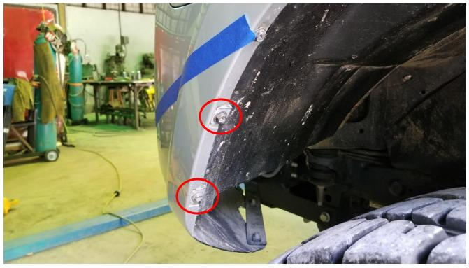
Using the 1" painters tape, make a diagonal line from the edge of the remaining OEM bumper cover down the fender liner as shown. The final cut of the fender liner is up to your discretion. Please use this picture as a reference.
