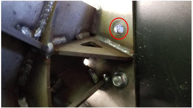
Remove the High Clearance side protection. Center punch and drill the marked holes. Use a ½" drill bit to allow for some adjustability. Do the same for the opposite side. \*\*To help prevent rust, clean the area of shavings and touch up the newly drilled holes with the provided black touch up paint.\*\*
