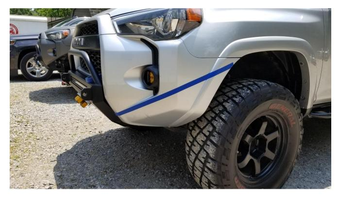
Using the Dremel with ripsaw or high speed cut-off wheel, carefully make the cut on the **bottom edge** of the painters tape from point to point as shown. Always use protective eye wear when cutting plastic.
