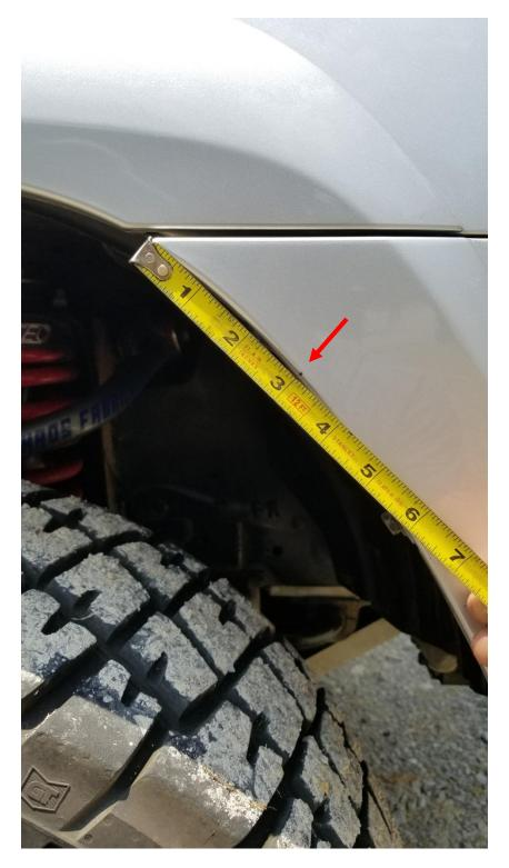
Now, measure from the bottom of the wing tip of the Slimline Hybrid and make a small mark at 2-1/4" from the bottom up, as shown.
