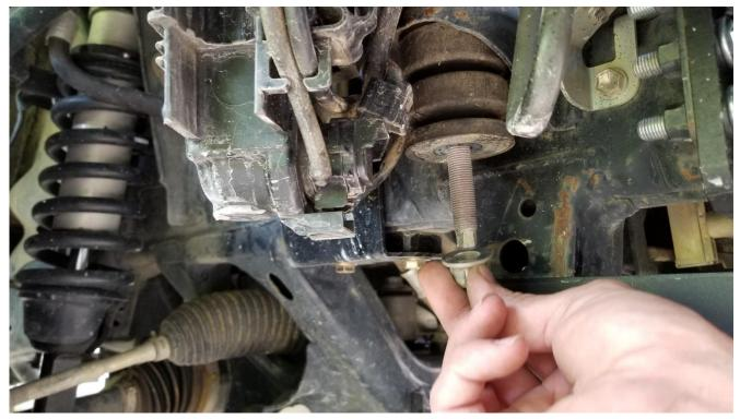
Simply slide the cover over the bottom of the washer bottle lining up the tab with the body mount bolt. Hold the washer bottle cover in place while torqueing the body mount bolt to 30-35 ft/lbs.
