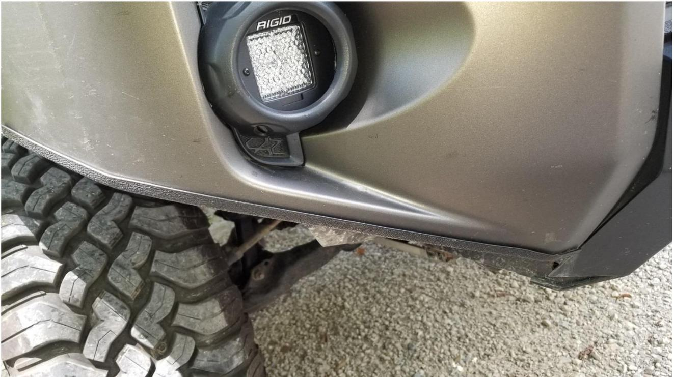
Reinstall the Stage 2 High Clearance on both sides for the final fitment. Use the provided 3/8"-16 flange nuts and the 3/8" bolts you removed from the side brackets earlier.
