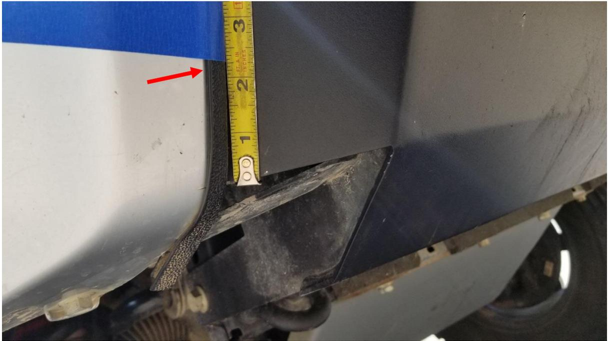
Using this newly created line, carefully place your 1" wide painters tape as straight as possible. **The bottom edge of the tape should be used to line up the marked points.** It is helpful to utilize the straight edge under the fog light as a guide when connecting each newly created point.
