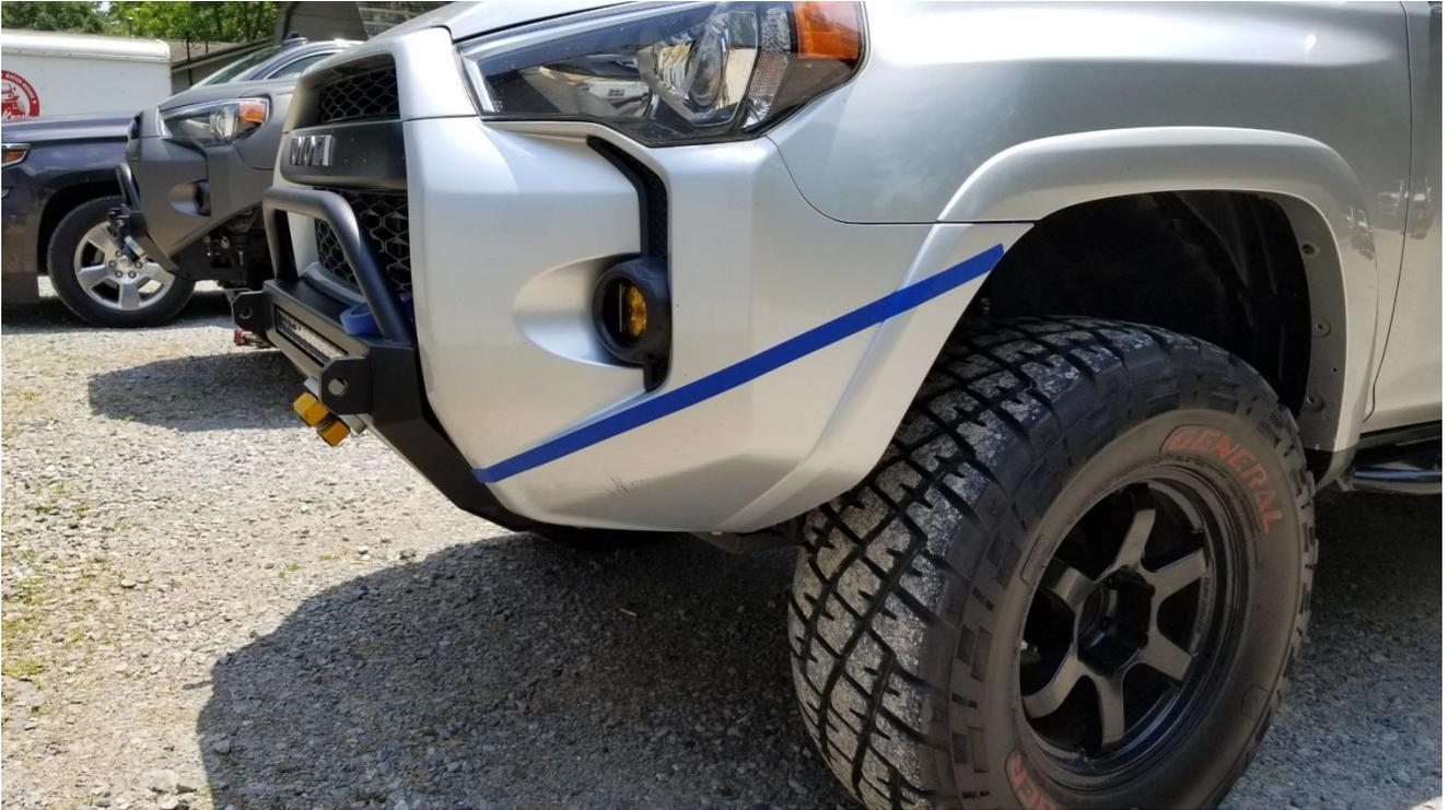
Using the Dremel with rip saw or high speed cut-off wheel, carefully make the cut on the **bottom edge** of the painter's tape from point to point as shown. **Always use protective eye wear when cutting plastic.**
