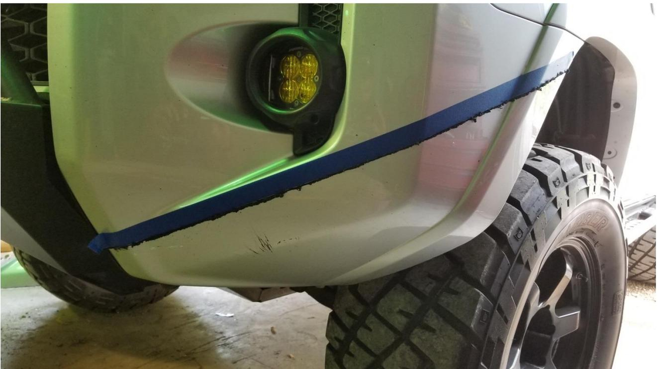
Once the cut is complete, remove the two 10mm screws from the fender liners to release the cut plastic. Leave the top 10mm screw in place.
