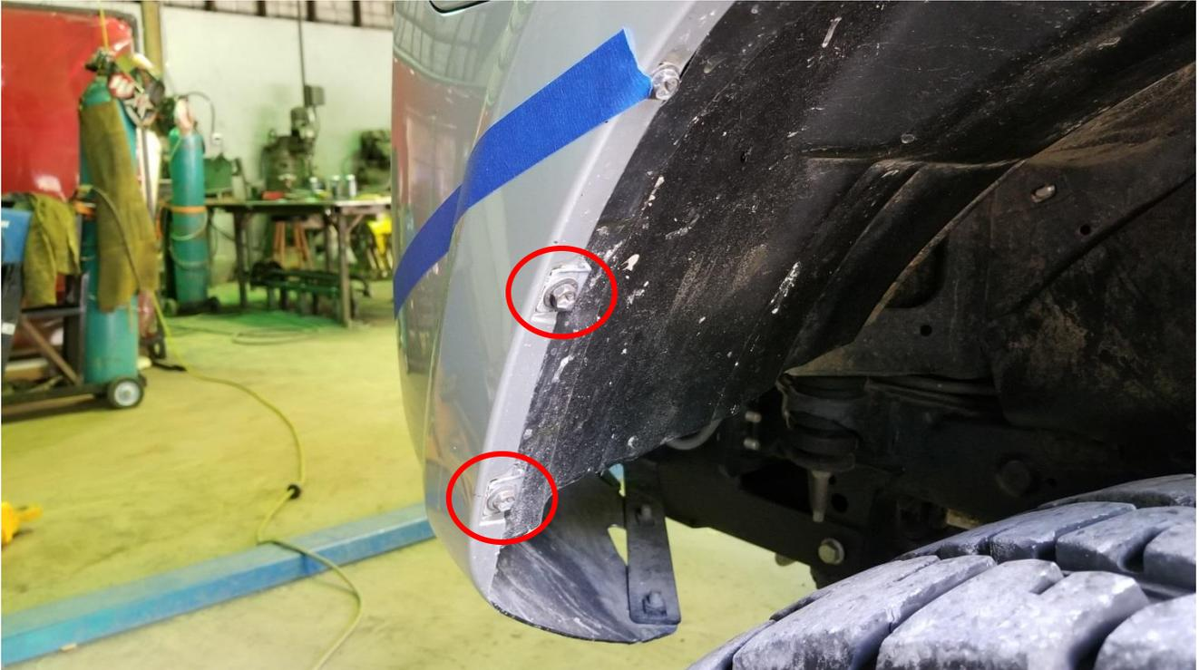
Using the 1" painters tape, make a diagonal line from the edge of the remaining OEM bumper cover down the fender liner as shown. The final cut of the fender liner is up to your discretion. Please use this picture as a reference.
