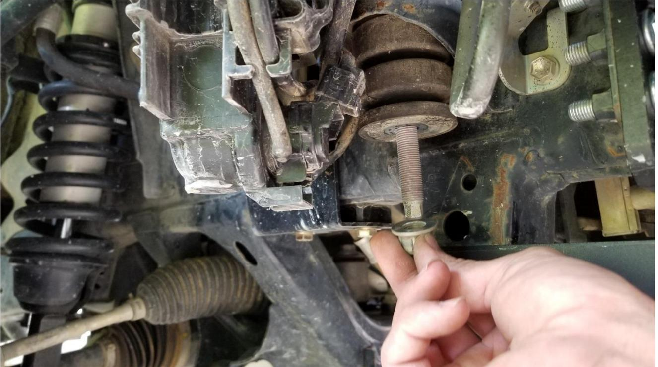
Simply slide the cover over the bottom of the washer bottle lining up the tab with the body mount bolt. Hold the washer bottle cover in place while torquing the body mount bolt to 30-35 ft/lbs.
