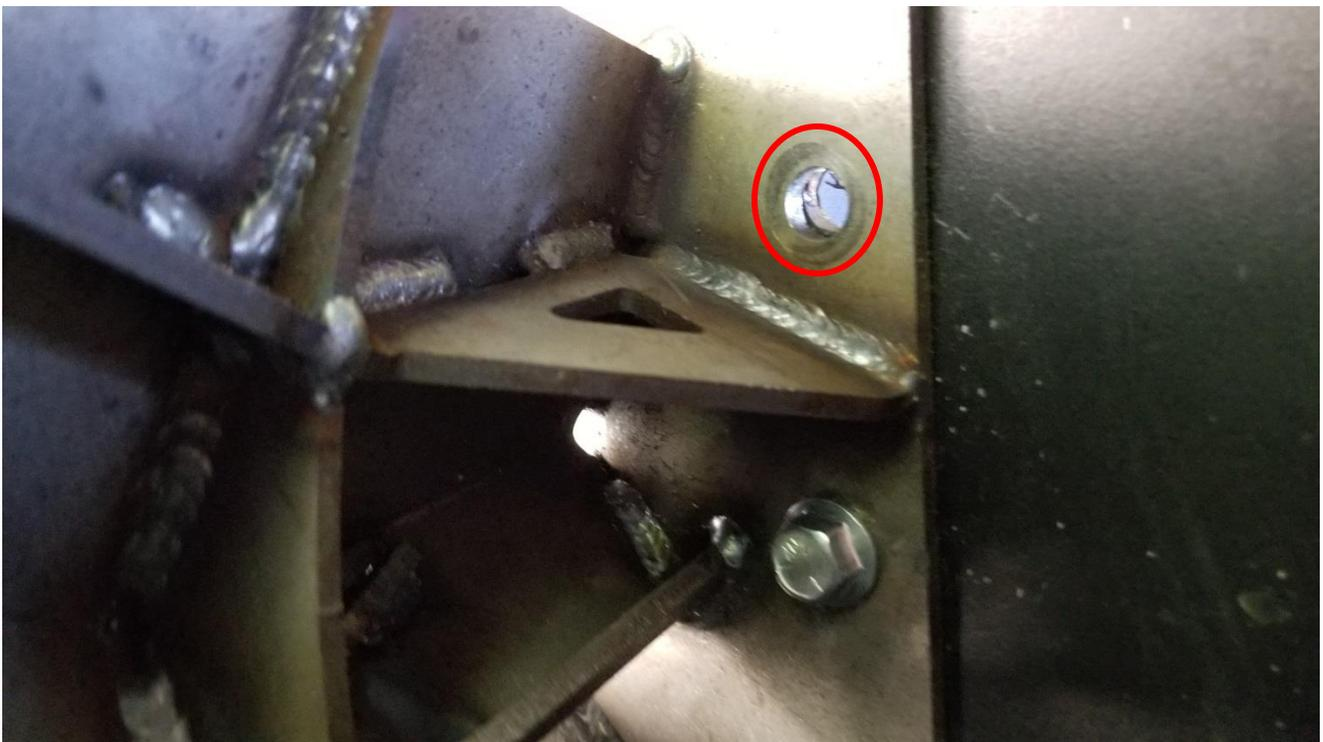
Remove the High Clearance side protection. Center punch and drill the marked holes.
