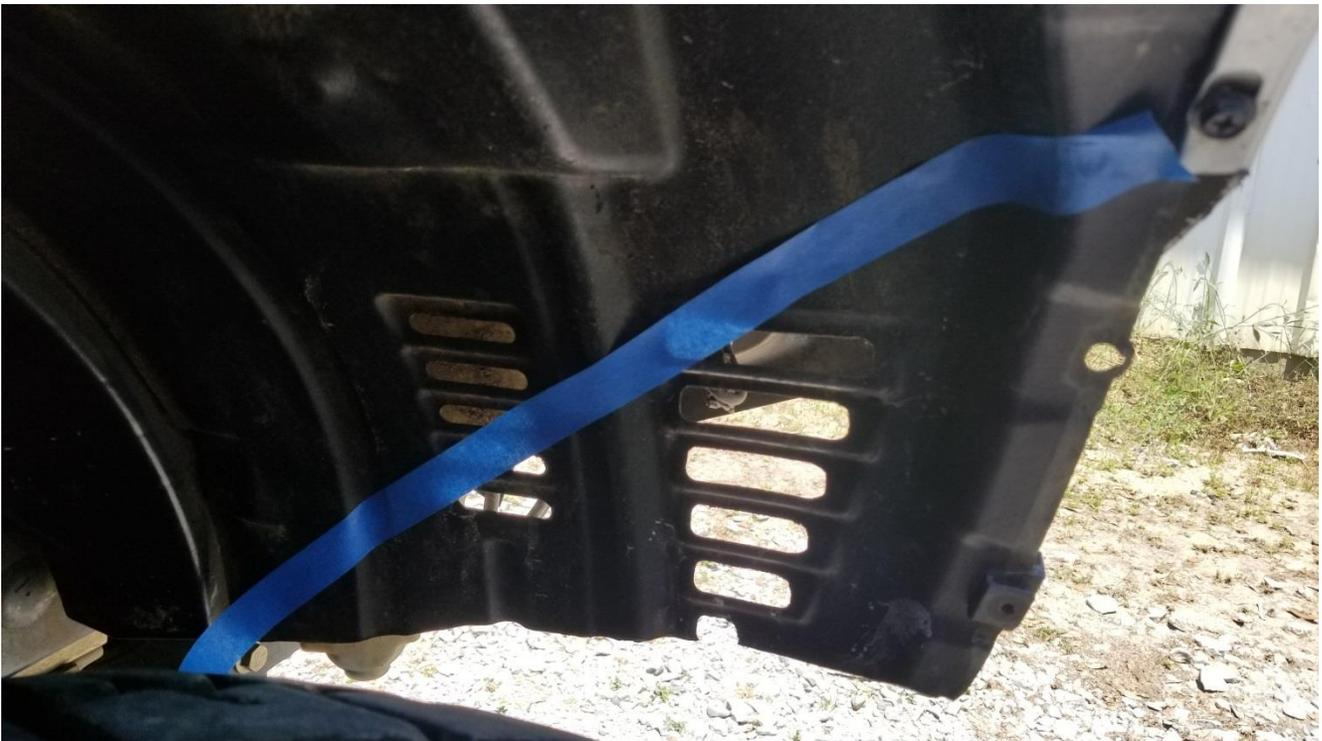
Remove the m12 (17mm head) from the lower radiator support. Lift the High Clearance side protection into place to mark and drill for new holes. (New Slimline Hybrids already have these holes in place, no drilling required). Once proper alignment is achieved, reinstall the m12 bolt to hold the side protection in place. Also install the 3/8 bolt in the pre-tapped hole from the top. The top bolts are accessed from the engine bay. Mark the two holes to be drilled circled in red.
