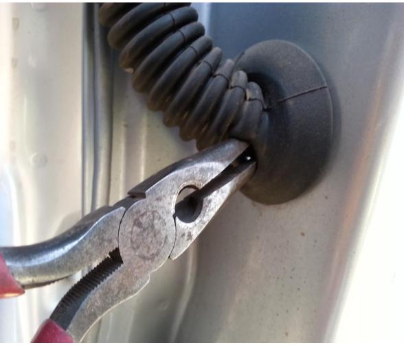
Poke a hole in the factory door grommet as shown.
