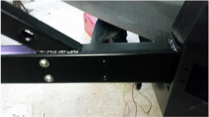
Install your license plate and bracket with ¼" button head bolts. Connect the positive wire to the license plate wire in the harness extension and run the wire the length of the swing arm to the grommet near the spindle.
