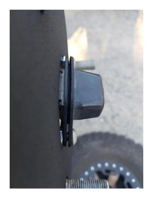
You'll also notice that the camera back plate has been cut so that you can easily bend the camera into the position that best suits your install. This will help keep he camera focused directly behind you instead of off into the distance.
