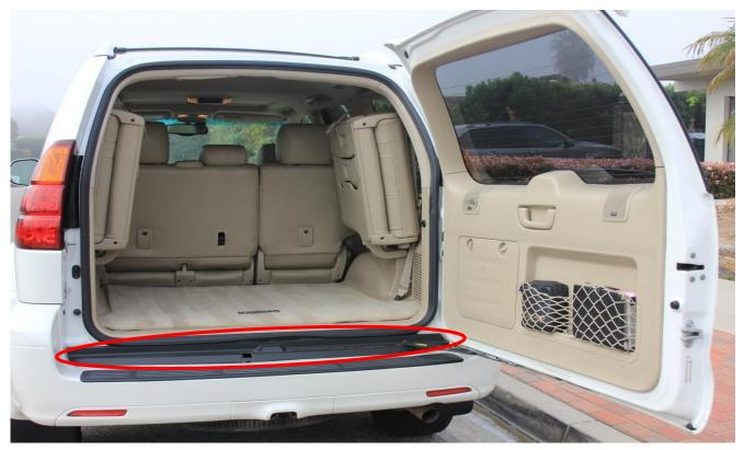
Now you are ready to remove the bumper skin. Pull down and away at each corner of the bumper. IF YOU FEEL AS IF THE BUMPER IS NOT LOOSE ENOUGH OR DOESN'T SLIDE OFF EASILY, STOP AND MAKE SURE THERE ARE NO BOLTS REMAINING.
