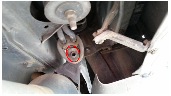
Finally remove this 10mm/Philips screw. It will be located within the fender well in the very corner of the bumper skin nearest the tire.
