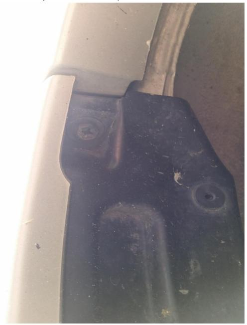
Next, open the back door and remove this 10mm bolt holding the back doors stopper. Lift the stopper arm off of the bolt. Now you will be able to gently pry off the black plastic cover to reveal some more push pins and screws still holding the bumper skin
