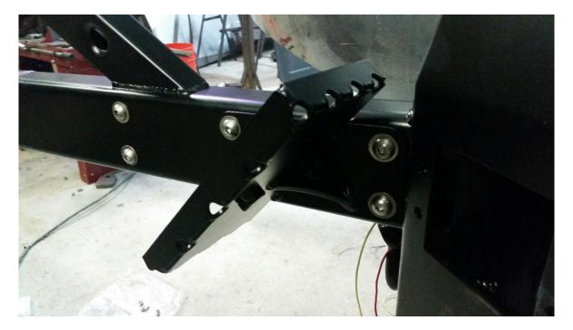
Install the upper hi lift mount above the heim joint using the supplied  $\frac{1}{4}$ " bolts.
