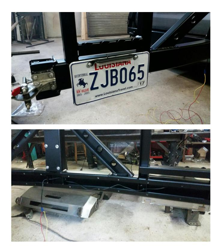
Also take this time to run your backup camera extension wires up the swing arm into the wheel mount area. Reconnect the extension harness camera wires to the section of plug and wire snipped off the oem harness. It is best to "stagger" your butt connectors so that they will still fit through all passages. Your remaining wire is for auxiliary backup lights wherever you should choose to put them. Keep this wire available to you for later.
