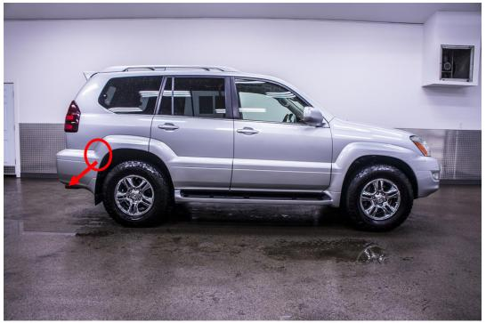
Reinstall the towing harness in this location. Simply run the OEM bolt through the original bolt hole backwards and into a pre-tapped hole on the backside of the cross member.
