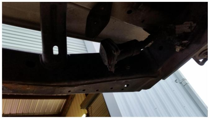
Ensure that the factory welds are smooth across the frame rails. Grind down any welds that prevent the 3/8" brackets from seating flat against the frame.
