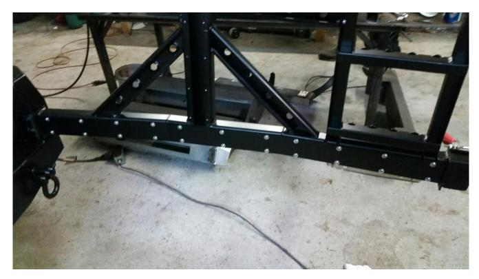
If you purchased the optional high lift mount, install the lower bracket using the remaining 3/8" bolts into the swing arm as shown. Otherwise, just install the bolts without the bracket.
