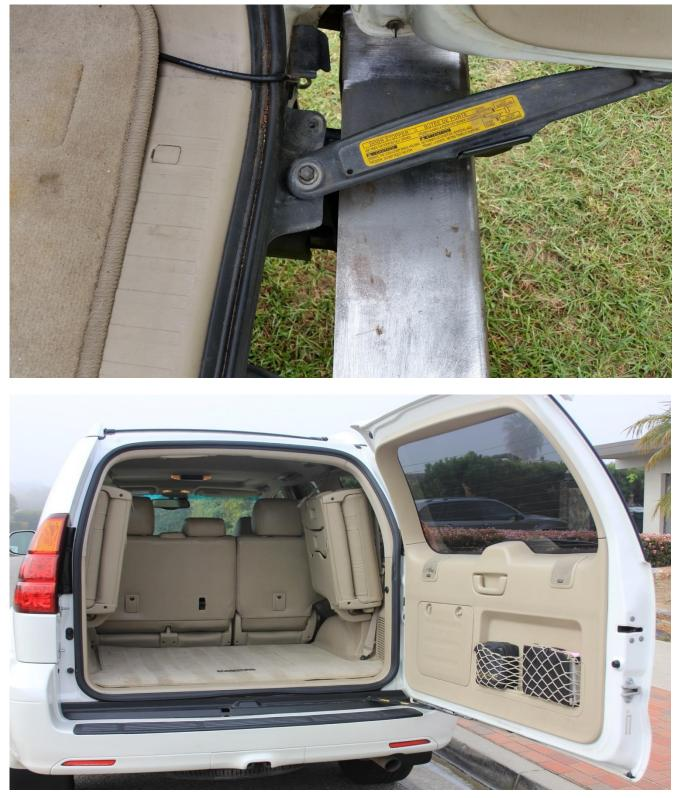
CONGRATULATIONS! You've just successfully installed your Southern Style OffRoad GX470 rear steel bumper. There should be some gap between the bumper and the body of the truck to allow for flex during extreme trail riding. This is normal.
