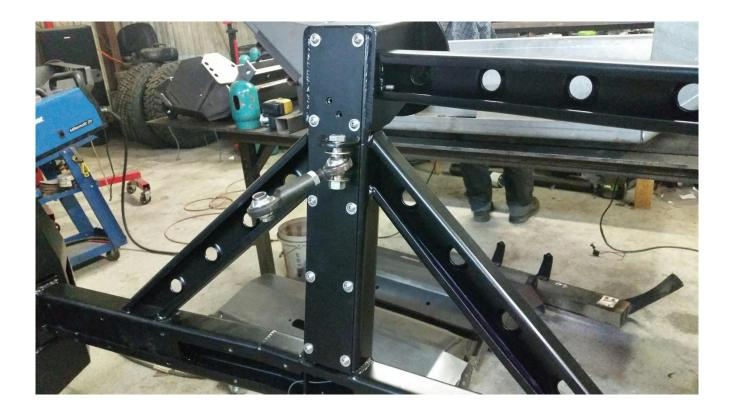
After all wires and harnesses have been run and fully tested for functionality. Install the large swing arm back plate using the remaining ¼" button head bolts and washers.
