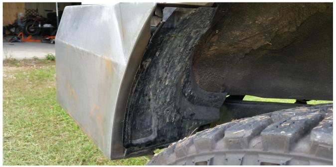
Reinstall locking door arm with or without plastic trim. The bumper was not specifically designed to reaccept the black plastic trim but it does still fit and fill the gap nicely.
