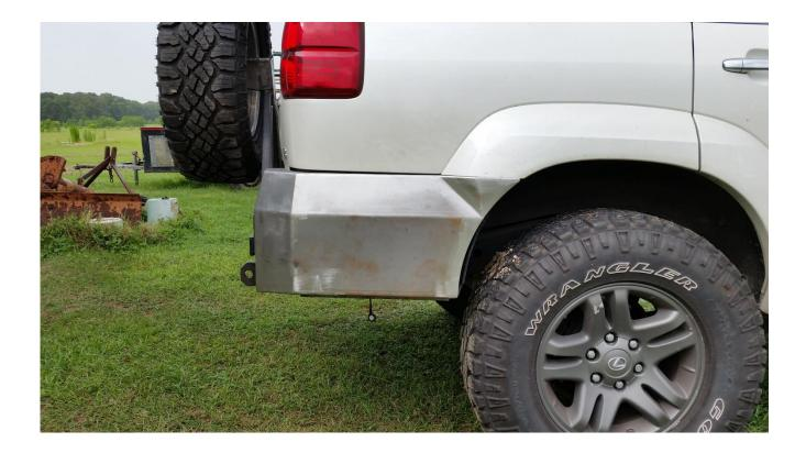
Trim your fender plastic to roughly match the outline of your new steel bumper, tuck the remaining fender liner behind the steel lip.
