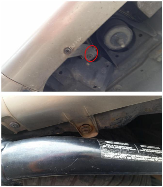
Slide the muffler off of its hanger using a little WD-40. You can let the tip hang. We will be reinstalling it or you can take this opportunity to chop your exhaust for better clearance as it will be the lowest point and will not be protected.
