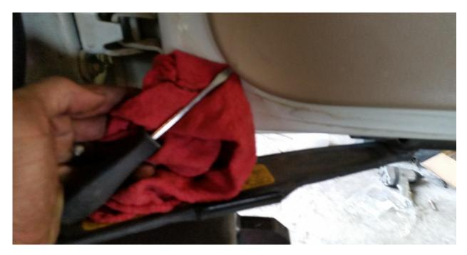
Once you feel as though all pins have been released, go to the top corners of the door panel and gently pull the corners from under the window trim.
