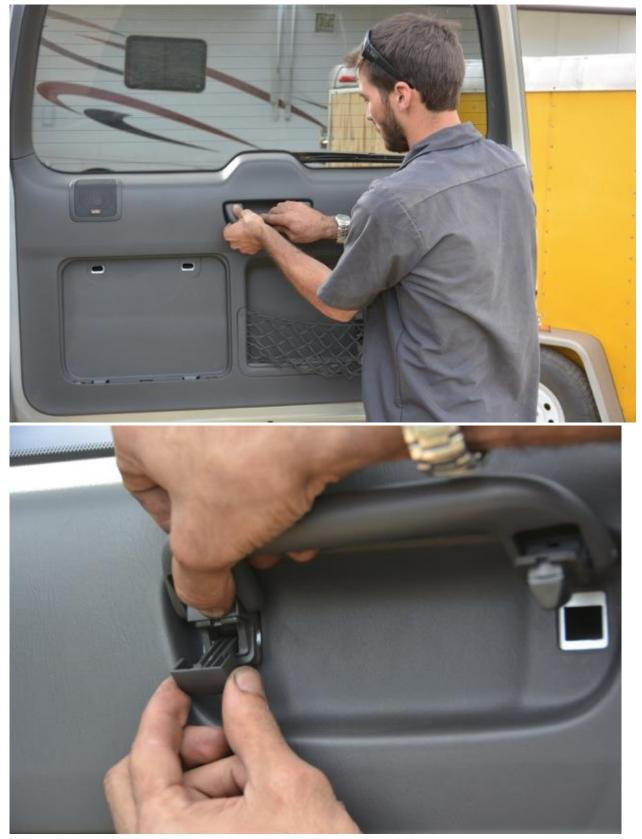
Continue on by removing the tool kit and door handle from interior of back door.
