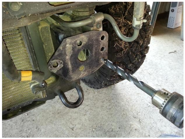
Using a 12mm socket, remove the bolt holding the pressurized fluid line bracket on both driver and passenger frame rail.
