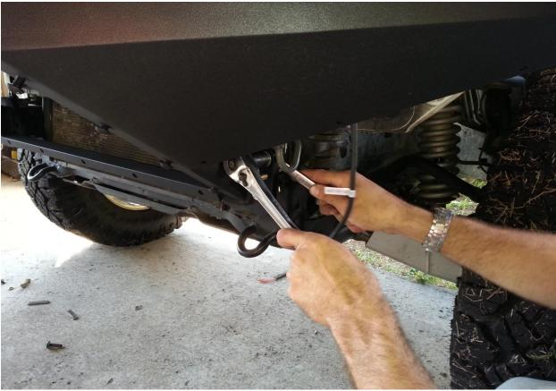
Remove the two 12mm bolts securing the factory skid plate.
