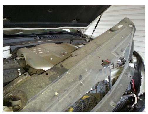
After removing the engine covers, you will also need to remove the remaining clips holding the front bumper cover onto the truck. You will find these clips between the headlights near the grill area.
