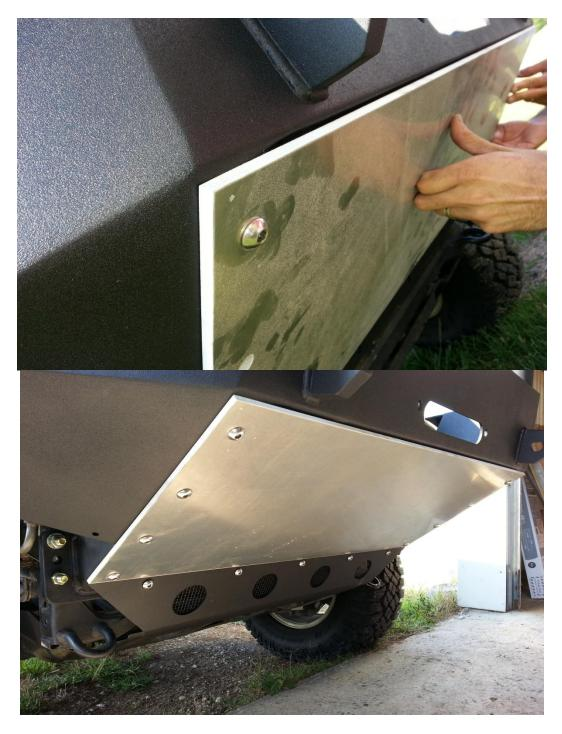
If ordered, install the sheet metal splash guards with the supplied  $\frac{1}{4}$ " button head bolts and washers. Also use a small amount of blue loctite on these threads to ensure no vibrations or bumps loosen the bolts.
