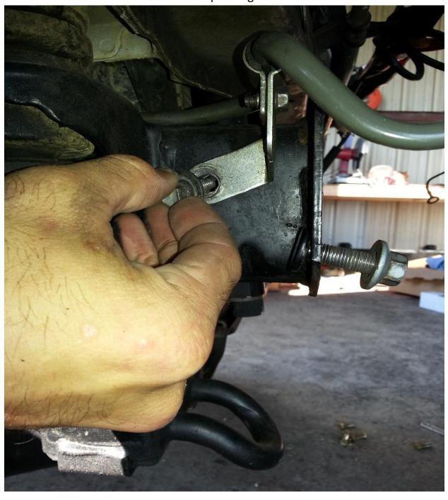
At this point, you may find it necessary to smooth out the OEM frame welds to ensure the new bumper bracket fits flush against the side of the rail. This may not be necessary for all vehicles.
