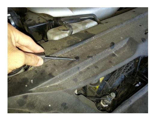
First, remove all the plastic clips holding the engine covers in place so that you may remove the covers for now. To do this, use a flat head screwdriver to pop the center section up. Once you have accomplished this, hold the clip at its base and pull it out of the mounting hole.
