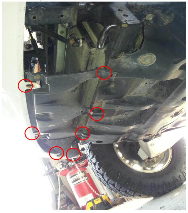
Remove the remaining clips and fasteners connecting the fender liner to the front bumper cover. You will want to wait until after the OEM bumper cover is removed before attempting to cut your fender liners out. This can be done with a sturdy pair of scissors. Carefully cut a straight line in the area highlighted below in the bright green circle. If done carefully, reinstallation of fender liners can be achieved by using industrial strips of Velcro or similar locking fasteners for a clean look.
