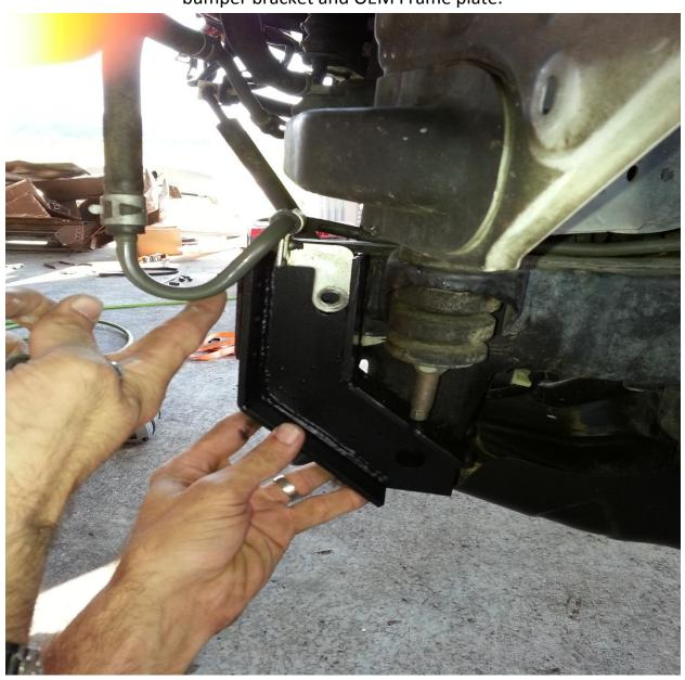
You can see here that we only left a single bolt on the outside edge on both the driver and passenger side. We found it much easier to locate the holes on the bumper to only one bolt on each side. The other bolts can be installed after getting the bumper lined up.
