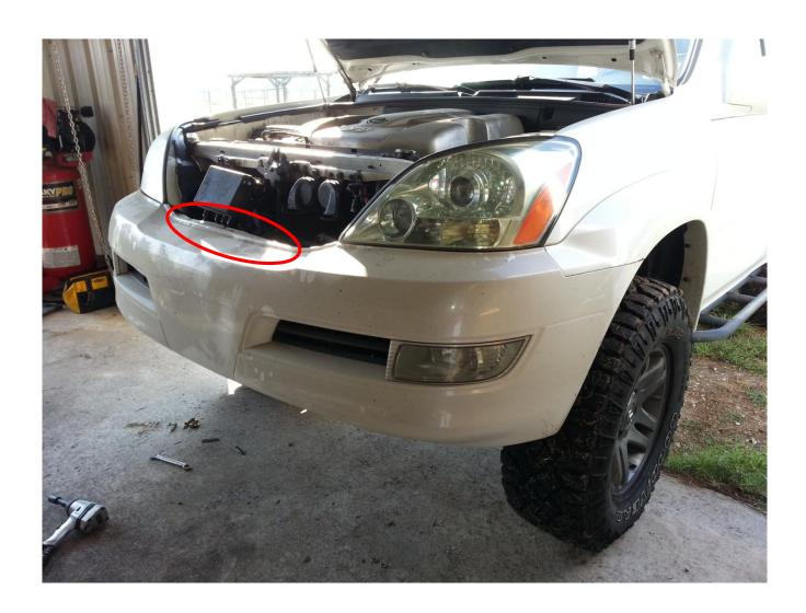
Remove every 10mm bolt on the underside of the OEM bumper cover. This will help to free up the plastic fender liners for removal in the next step.
