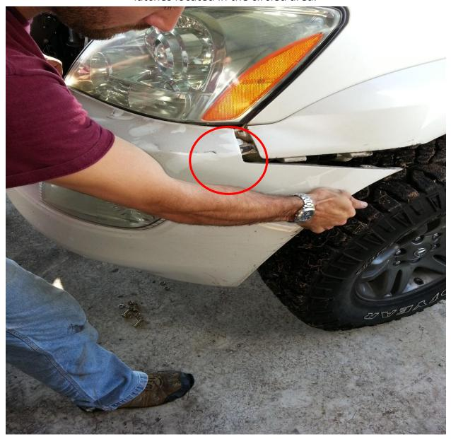
After disengaging these latches the bumper should start to easily "peel" off.
