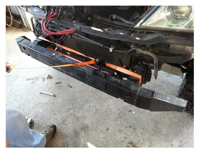
You will find it necessary to increase the tension on the crash horns until the center section starts to loosen on the bolts. Under the correct tension, it should be easy to remove and reinstall the center section.
