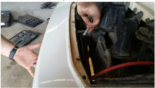
If you purchased the optional shackle mounts, measure approximately 2 inches from the center vertical slat inwards towards the center of the bumper. Make a mark, measure an additional ¾" for the width of the shackle mount. Cut the horizontal slat in the oem bumper to make clearance for the shackle mounts.
