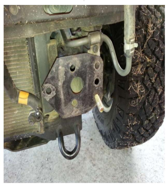
Install the hidden winch bumper using the provided grade 8 hardware as shown. Do not install the optional shackle mounts yet. Don't forget the 2 bolts inside and underneath the frame rail section.
