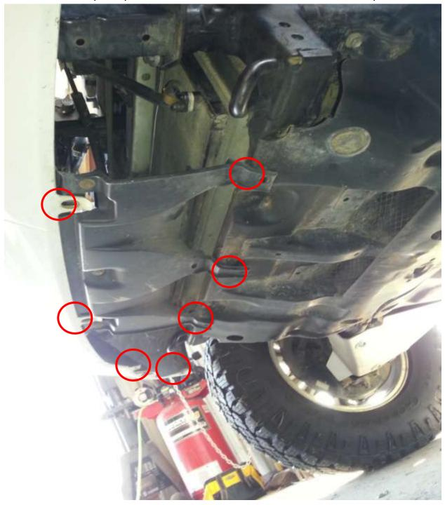
Remove the remaining clips and fasteners connecting the fender liner to the front bumper cover.
