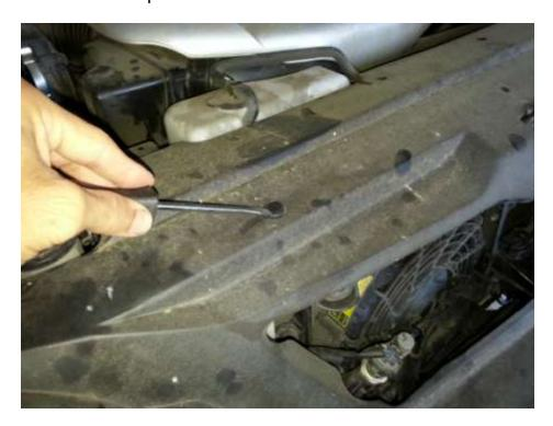
First, remove all the plastic clips holding the engine covers in place so that you may remove the covers for now. To do this, use a flat head screwdriver to pop the center section up. Hold the clip at its base and pull it out of the mounting hole.
