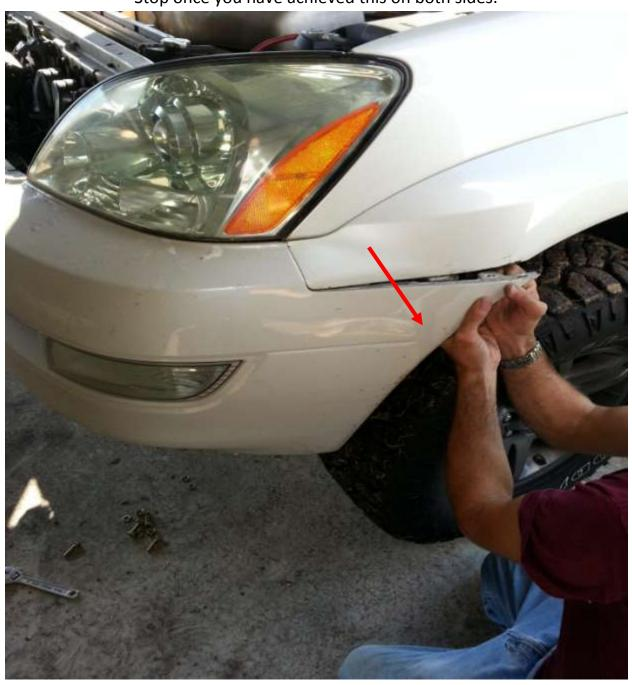
Next, stand in front of the vehicle on the same side that you just started removing the bumper cover. By pulling downward and towards you, disengage the large plastic latches located in the circled area.
