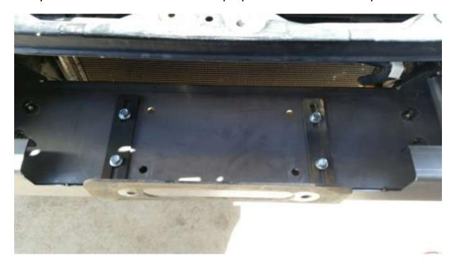
Place your oem bumper cover back over the hidden winch. Make sure it snaps into the sides, but no bolts are needed. At this point you'll want to slide the fairlead forward so that it is making contact with the back of the oem bumper. Tighten the fairlead mount down. Also, using a sharpie marker or similar, trace the fairlead holes onto the back of the oem bumper to be cut out and drilled.
