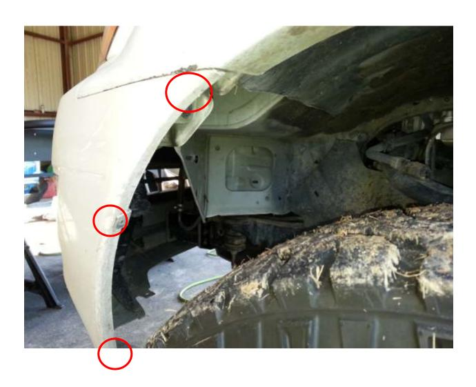
Before continuing, be certain that all plastic clips, screws, and bolts holding the OEM bumper cover onto the truck have been removed. To get started, pull down and out at the corner indicated in the picture. This may take more force than anticipated. The OEM bumper is designed to latch to the fender even without any hardware holding it.
