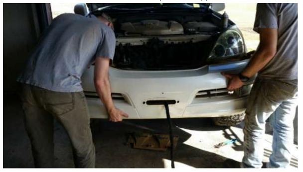
Install your fairlead by carefully holding the nut behind the fairlead mount while threading the bolt through the front of the fairlead.
