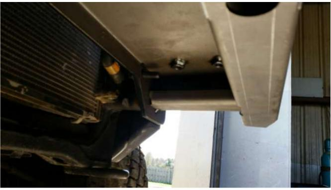
Loosely install the fairlead mount so the proper distance to the bumper can be set.
