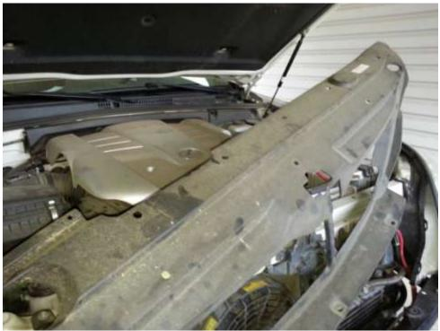
After removing the engine covers, you will also need to remove the remaining clips holding the front bumper cover onto the truck. You will find these clips between the headlights near the grill area.
