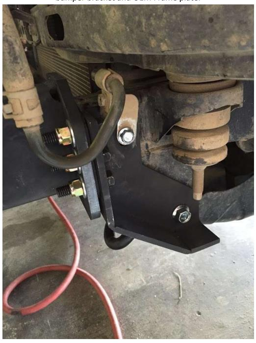
You can see here that we only left a single bolt on the outside edge on both the driver and passenger side. We found it much easier to locate the holes on the bumper to only one bolt on each side. The other bolts can be installed after getting the bumper lined up.
