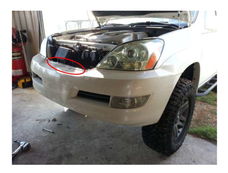
Remove every 10mm bolt on the underside of the OEM bumper cover. This will help to free up the plastic fender liners for removal in the next step.
