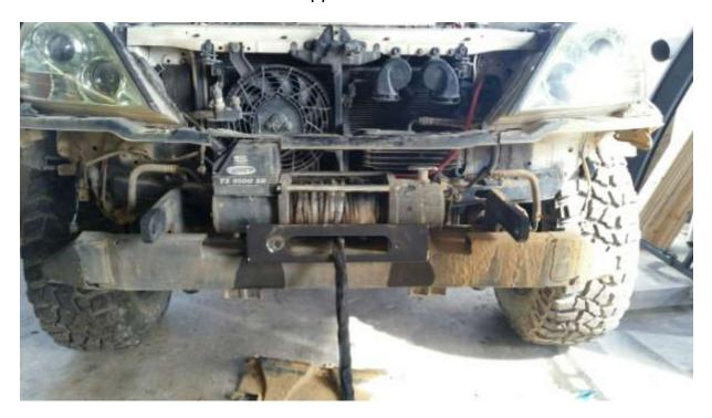
Pass the winch line through the oem bumper and carefully reinstall making sure your previous marks and cuts line up with the hidden winch. Reinstall your bumper using the oem hardware and clips where applicable.
