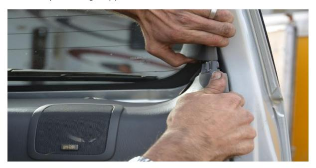
At this point, the door panel should be free, if it is not, double check that all pushpins have been released and finally pull the door panel away from the door.
