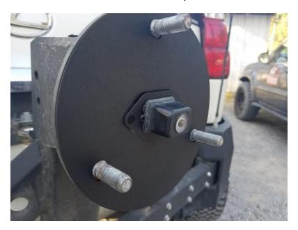
Sandwich the camera between the back plate and the adapter plate
