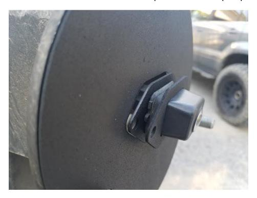
Tighten the provided ¼" button head bolts and nuts so that the camera is snug.
