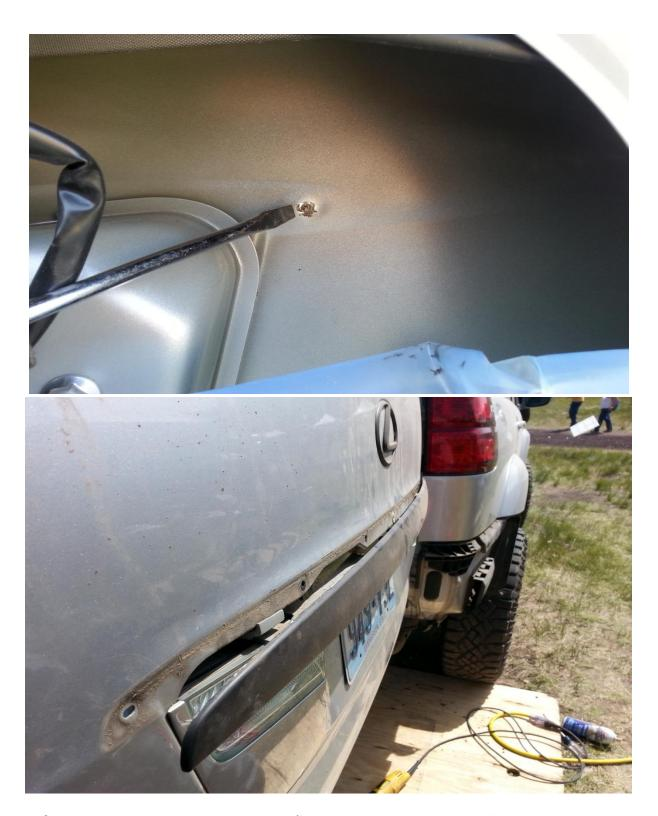
After removing this trim piece, you'll gain access to two small bolts holding the backup camera into place. Remove these bolts.
