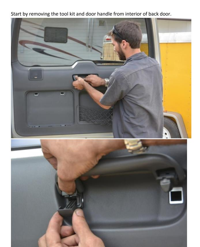
After removing plastic pins on both side of the handle, pull down and away to remove handle from frame of door
