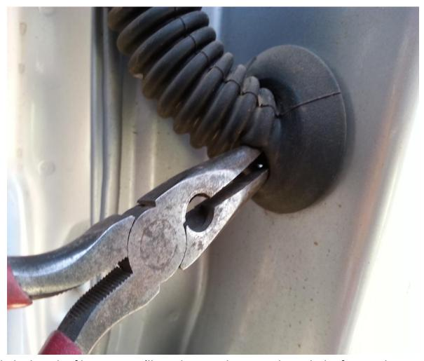
Mark the length of harness you'll need to run the wires through the factory door grommet and to the 4 OEM wires you just cut. Use the heat shrink around the supplied wire harness. Leave approximately 8-10 inches of wire and plug hanging out of the door grommet.
