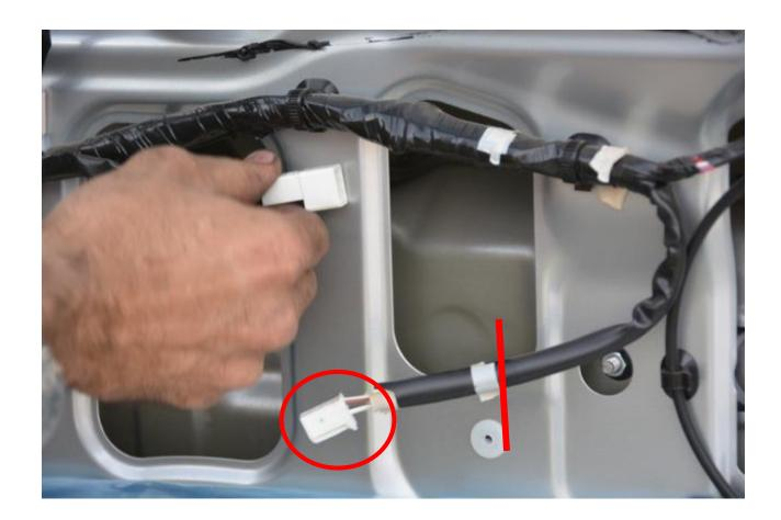
Cut the OEM wiring harness at the point indicated in the picture above. It is important that you make this cut so that there are 4 wires and not 3. One of those wires is a shielded cable that splits off into 2 near the electrical connector. Once again, make sure you make the cut where there will be 4 wires on both sides of this cut. You may need to trim away some of the black protective loom.
