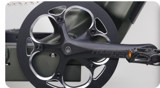
Right pedal (1) tightens clockwise
