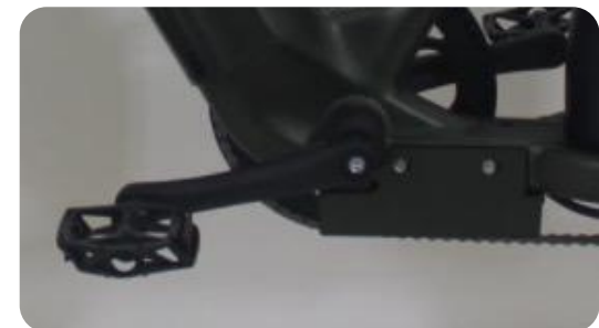
Left pedal (2) tightens counterclockwise
