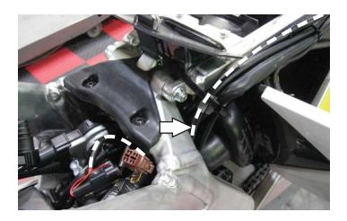
5 Route the PC6 harness along the left side of the sub-frame and go towards the throttle body. Use the stock cable ties to secure the PC6 harness to the stock wiring harness.
