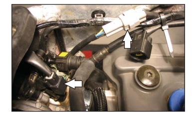
8 Plug the PC6 wiring harness in-line of the stock wiring harness and injector.
