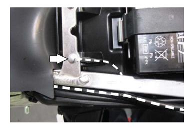
4 Attach the ground wire from the PC6 to the sub-frame bolt.
