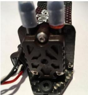
**Install the fluid delivery line(s) to the smoke pump.**
