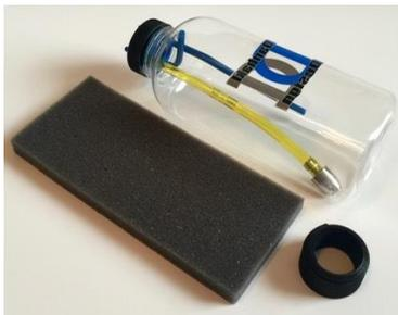
If you prefer to build your own tank, it should be assembled with three lines: a line for the non-filtered pickup (clunk), a vent line and a fill line. Per the Fourtitude ARF tank pictured, a fill line that is bent toward the tank floor facilitates filling as well as draining the tank.
