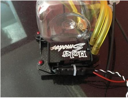
pilot holes and mount the pump. Take care to allow a slight amount of movement. Vibration isolation is lost if the screws are fastened too tight compressing the grommet.
