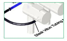
**Secure and route all tubing connections.** Take care to route the high temperature tubing away from the hot mufflers preventing chaffing/rubbing. Secure all tubing connections with a small zip tie.
