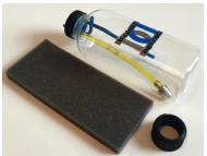
If you prefer to build your own tank, it should be assembled with three lines: a line for the non-filtered pickup (clunk), a vent line and a fill line. Per the Fourtitude ARF tank pictured, a fill line that is bent toward the tank floor facilitates filling as well as draining the tank.
