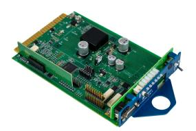
• INTEGRATED CONFIRMATION technology powers IC enabled DETOC series TOMAR Strobecom II detectors to be powered and controlled over the standard preemption detector cable. No additional power supplies, mounting, programming, or wiring required.
