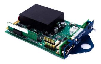
• INTEGRATED CONFIRMATION technology powers IC enabled DETOC series TOMAR Strobecom II detectors to be powered and controlled over the standard preemption detector cable. No additional power supplies, mounting, programming, or wiring required.
