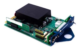
• INTEGRATED CONFIRMATION technology powers IC enabled DETOC series TOMAR Strobecom II detectors to be powered and controlled over the standard preemption detector cable. No additional power supplies, mounting, programming, or wiring required.
