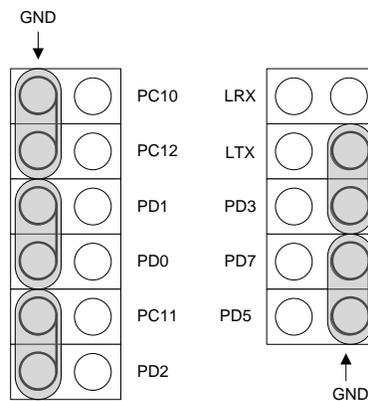
Figure 2: Default Jumper Placement
