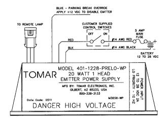
The Model 401-1228-PRELO Emitter Power Supply is designed for mounting on a sturdy flat surface protected from rain, spills, excessive heat, and physical damage. It may be installed in the trunk of a car, the saddlebag of a motorcycle, or other similar protected location. This device may also be installed in the engine compartment of a vehicle as long as it is mounted to a sturdy, flat surface, as far away from the engine as possible.
