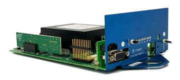
• INTEGRATED CONFIRMATION technology powers IC enabled 4000 series TOMAR Strobecom II detectors to be powered and controlled over the standard preemption detector cable. No additional power supplies, mounting, programming, or wiring required.
