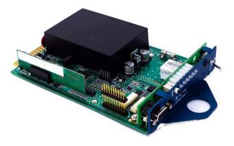
• INTEGRATED CONFIRMATION technology powers IC enabled 4000 series TOMAR Strobecom II detectors to be powered and controlled over the standard preemption detector cable. No additional power supplies, mounting, programming, or wiring required.
