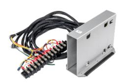
The TOMAR 1881 Card Cage can be used for simple installation of a TOMAR STROBECOM II optical signal processor (OSP) card when a traffic signal cabinet does not have an available card slot. The 1881 Card Cage will work with 2000, 3000, 4000, or OSPOC series STROBECOM II OSP's, in both 2 and 4-channel. The 1881 includes a harness to operate channels A, B, C, & D, and the rack provides 120 VAC to power the OSP.
