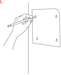
Position mounting template on the wall at the desired location. Make sure the unit is level and mark the drill holes. 2.
