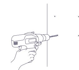
Remove mounting template. If mounting on drywall, use a 1/2" bit to drill pilot holes where the markings were made.
