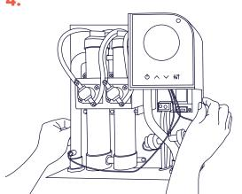
Remove front cover of heater. Align screws with the mounting holes on the back of heater and gently place it onto the wall. Make sure the unit is secure before letting go.
