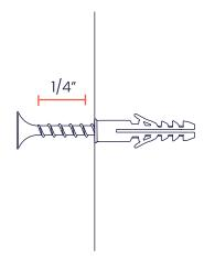
Use (4) drywall anchors and (4) mounting screws. Insert the anchors into the drilled holes, then thread screws into anchors. Do not thread screws all the way down. Leave them out about ¼".
