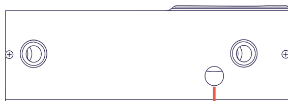
3/4" punchout with Romex connector
