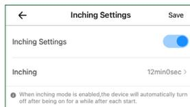
4. Enable Itching Settings and set Itching to 12 min. This will tell the device to turn off 12 minutes after each time it is started.
