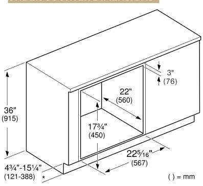
**NOTICE:** The cabinet base must be flat and capable of supporting a weight of at least 142 lbs (64.1 kg).
