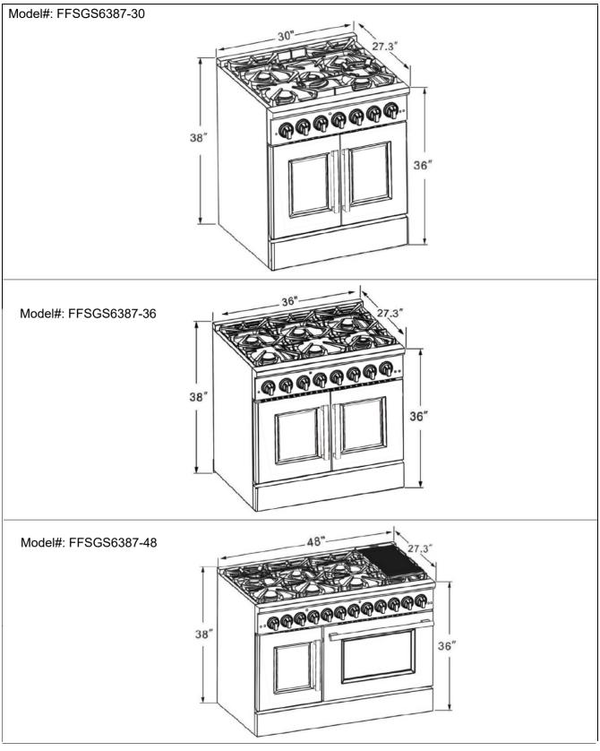
This range may be installed directly adjacent to existing countertop-height cabinets (36" or 91.5 cm from the floor). To achieve the best look, the cooktop should be level with the cabinet countertop. This can be accomplished by raising the unit using the adjustment spindles on the legs.
