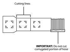
2 If a longer drain hose is required, you can add up to 42" (1.1 m) of length, for a total of 10 ft. (3.01 m) to the factory installed hose. Use 5/8" or 7/8" inside diameter hose and a coupler to connect the two hose ends. Secure the connection with screw-type hose clamps.
