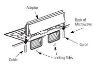
Push in securely until it is in the lower locking tabs. Take care to assure that the damper hinge is installed so that it is at the top and that the damper swings freely.
