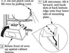
3 Insert a self-aligning screw through top center cabinet hole. Temporarily secure the oven by turning the screw at least **two full turns** after the threads have engaged. (It will be completely tightened later.) **Be sure to keep power cord tight.** Be careful not to pinch the cord, especially when mounting flush to bottom of cabinet.
