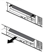
Slide the top of the new charcoal filter into the top of the filter cavity.
