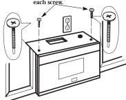
Tighten the outer two screws to the top of the microwave oven. (While tightening screws, hold the microwave oven in place against the wall and the top cabinet.)
