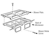
Remove the screw that holds the blower plate to the microwave. Remove and save the screw holding the blower motor to the microwave. 2 Carefully pull out the blower unit. The wires will extend far enough to allow you to adjust the blower unit.
