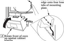
3 Insert a self-aligning screw through top center cabinet hole. Temporarily secure the oven by turning the screw at least **two full turns** after the threads have engaged. (It will be completely tightened later.) Be sure to keep power cord tight. Be careful not to pinch the cord, especially when recent if furth to hottom of solving.
