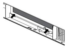
Reinstall the vent by sliding the bottom of the vent into place. Push the vent top into position and slide right into place. Replace the two vent mounting screws located on top of the microwave using a #1 Phillips screwdriver.
