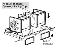
CAUTION: Do not pull or stretch the blower unit wiring. Make sure the wires are not pinched, and that they are properly secured.
