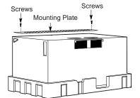
5 Remove the screws from each end of the mounting plate. This plate will be used as the rear wall template and for mounting. Reinstall the screws into the holes where they were removed.
