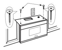
7 Tighten the outer two screws to the top of the microwave oven. (While tightening screws, hold the microwave oven in place against the wall and the top cabinet.)
