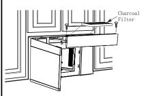
Remove the charcoal filter by pushing the top of the filter inwards,then pull it forward out from the unit.
