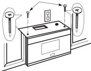
6 Tighten the outer two screws to the top of the microwave oven. (While tightening screws, hold the microwave oven in place against the wall and the top cabinet.)
