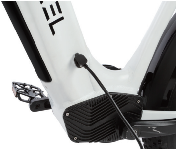
A. Recharge the battery on e-bike directly.
