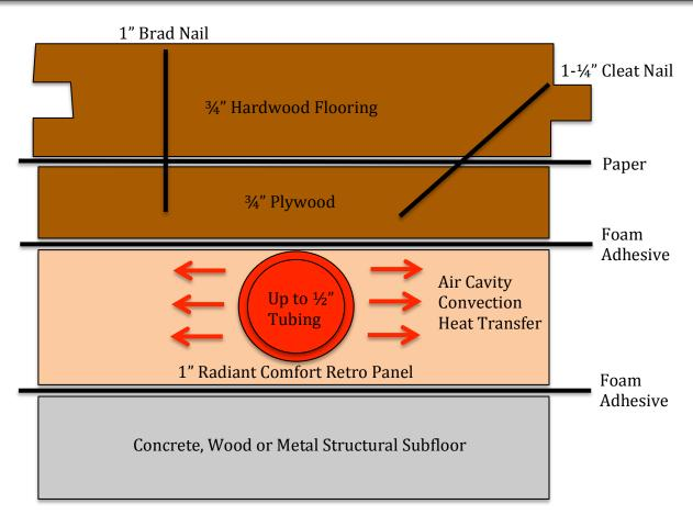
Required fasteners\*: Foam adhesive, 1" brad nails, 1-1/4" cleat nails
