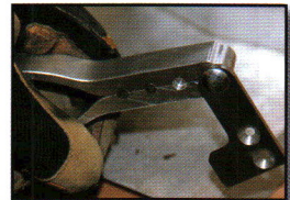
Figures 13 and 14: Use of mallet to tap sprue cutter and flat surface base of bullets.
