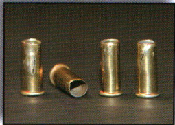
Figure 1: Split and Dented Cases
