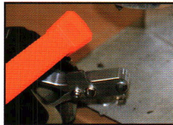
Figures 13 and 14: Use of mallet to tap sprue cutter and flat surface base of bullets.
