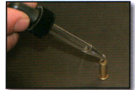
Figure 7: Putting drops of acetone into 22LR case to liquefy compound to allow for easier insertion into rim of case.
