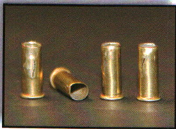
Figure 1: Split and Dented Cases
