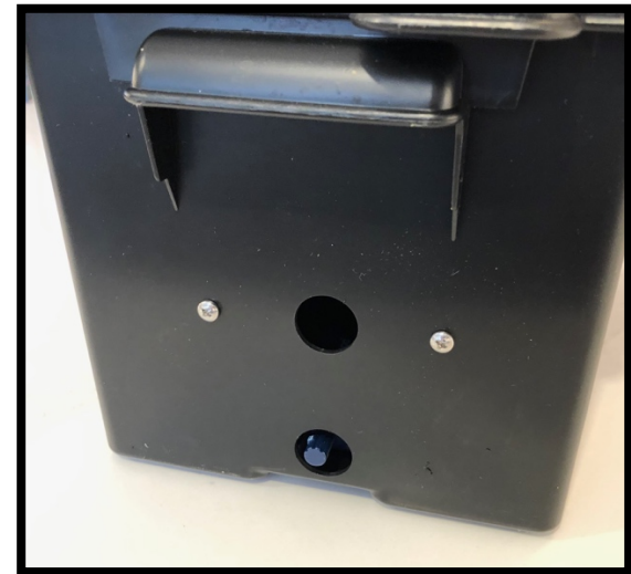
Protruding Blue Test Knob – rotate counterclockwise
