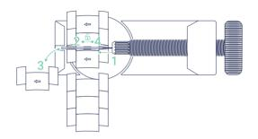
If the link bracelet does not quite fit, you can remove individual links and adjust it to the preferred size. To do this, insert a suitable watch tool into the opening (1) and loosen the locking pin in the direction of the arrows (2). Then you can remove/add bracelet links (3) to adjust the strap length. To close the bracelet, reinsert the pin in the opposite direction of the arrow and secure it (4).
