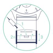
Insert a tool or another narrow object into the opening (1) of the slider. Release the locking mechanism (2) with a slight lever movement. You can then easily adjust the slider to the preferred size (3) and then lock it again (2).
