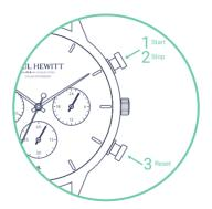
Press the start/stop pusher to start or stop the chrono's stopwatch (1)(2). Press the reset pusher to return the hands of the watch to their initial position (3).
