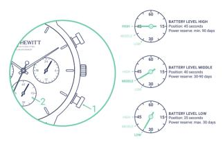
To display the battery charge level of your solar watch, press the reset button and hold it for two seconds. The hand of the stop second (2) will then show you the current charge level.
