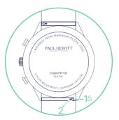
Press the bracelet lock inwards to unlock (1) and simultaneously move the bracelet away from the watch (2). Interchangeable bracelets can then be reattached in reverse order.
