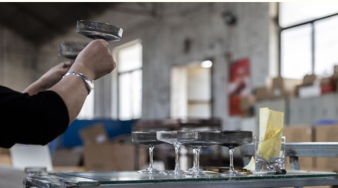
Inspection of a Ripple Champagne Saucer at our glass manufacturer in the Southwest of Beijing, Shanxi Province. As every single Ripple glass is mouth-blown, each piece is unique and none are 100% identical, as the glassblower influences the final result through the amount of glass and air pressure he or she uses during the blowing.
