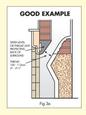
may cure the less serious cases. Bad cases often require further treatment. As well as helping air starvation a throat restrictor is an excellent means of making a room more comfortable by reducing the air induced up the flue and so reducing excessive ventilation.
