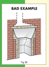
The void should be filled in and the throat reduced so that there is a smooth, streamlined entry into the flue as shown in Fig.3a and 3b. If the throat opening can be made adjustable for size it will be better still, as then the minimum amount of opening can be found to suit the 'pull' of the flue when the chimney is warm, and yet allow the full opening for relighting the fire when the chimney is cold.
