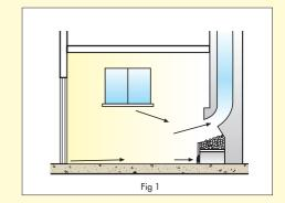
**REMEDY** It is necessary to allow more air into the room, but in a way that avoids unpleasant draughts, this is often difficult. The first step should be to see if it is possible to reduce the volume of air flowing up the flue so the 'demand' for air is less. An inspection of the throat over the fire may reveal a large throat without any attempt at streamlining and an even larger void beyond and at the sides - see Fig. 2a and 2b.
